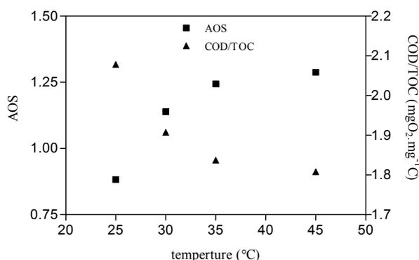
Figure 8.48: AOS and COD/TOC as function of operational temperature in photo-Fenton reaction.  $[H_2O_2]_i = 30 \text{ mg.L}^{-1}$ ,  $[Fe(II)]_i = 10$ , 50 min irradiation time and free pH evolution.
