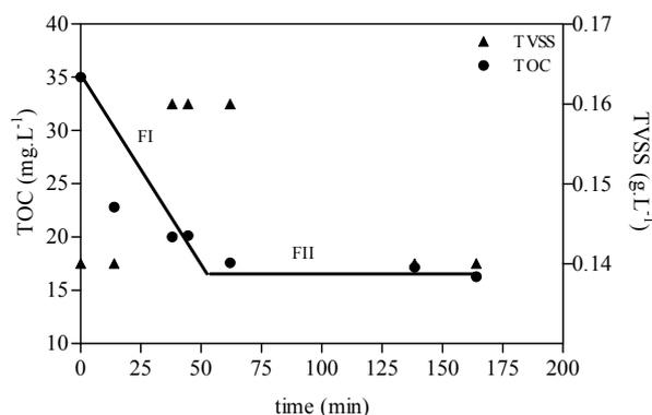
Figure 9.3: Evolution of TOC and TVSS as function of cycle duration, cycle duration 8 days and feed BOD<sub>5</sub>/COD= 0.21.
