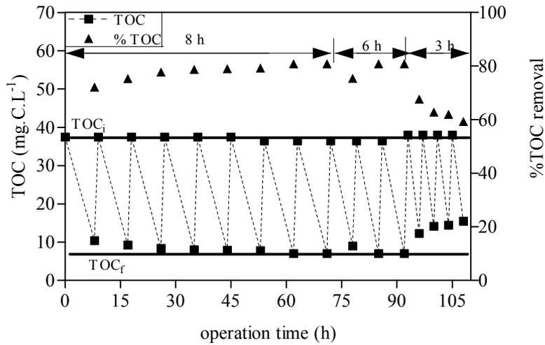
Figure 9.19: Evolution of initial organic carbon after feeding the reactor (TOC<sub>i</sub>), final organic carbon before next feeding (TOC<sub>f</sub>) and organic matter removal for each cycle (%TOC) as function of time, cycle duration 8, 6 and 3 h and feed BOD<sub>5</sub>/COD= 0.48.
