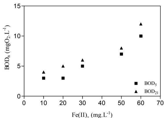
Figure 8.36 : BOD<sub>n</sub> as function of initial Fe(II) in multi lamps photo-reactor. [H<sub>2</sub>O<sub>2</sub>]<sub>i</sub>= 15 mg.L<sup>-1</sup>, 35 min irradiation time and free pH evolution.
