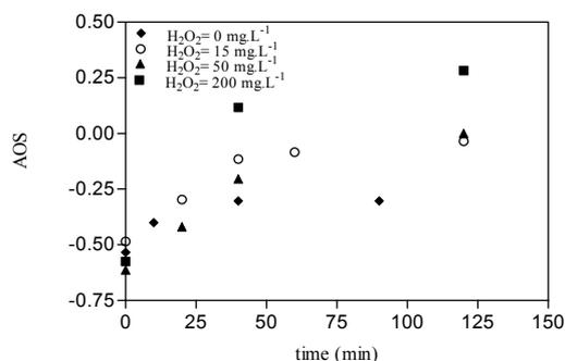
Figure 8.9: Evolution of AOS vs. reaction time for UVA/H<sub>2</sub>O<sub>2</sub> process at different initial H<sub>2</sub>O<sub>2</sub> concentrations in multi lamps reactor.
