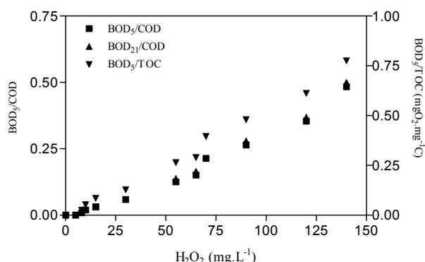
Figure 8.33: Evolution of BOD<sub>n</sub>/COD and BOD<sub>n</sub>/TOC as function of initial H<sub>2</sub>O<sub>2</sub> in multi lamps photo-reactor. [Fe(II)]<sub>i</sub>= 10 mg.L<sup>-1</sup>, 35 min irradiation time and free pH evolution
