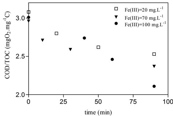
Figure 8.17: Evolution of COD/TOC as function of reaction time in UVA/Fe(III) process, for different initial Fe(III) concentrations in multi lamps reactor.
