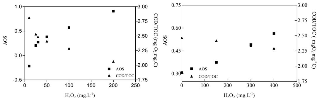
Figure 7.7: Evolution of COD/TOC and AOS as a function of initial H<sub>2</sub>O<sub>2</sub> concentration for DCP and POH in UV/ H<sub>2</sub>O<sub>2</sub> process. Reaction time 90 min.
