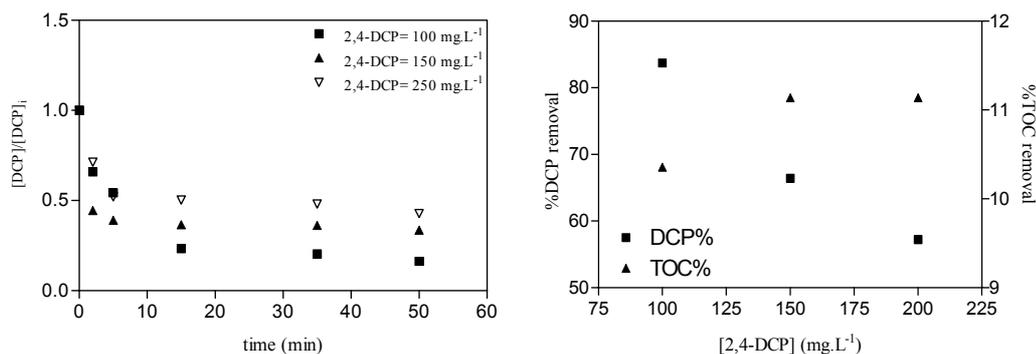
Figure 8.28: Evolution of DCP vs. irradiation time for different initial DCP for single lamp photo-reactor.  $[H_2O_2]_i = 30 \text{ mg.L}^{-1}$ ,  $[Fe(II)]_i = 10 \text{ mg.L}^{-1}$ .
