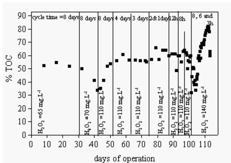
Figure 9.14: TOC removal as function of time at different initial H<sub>2</sub>O<sub>2</sub> used in photo-Fenton and cycle duration.
