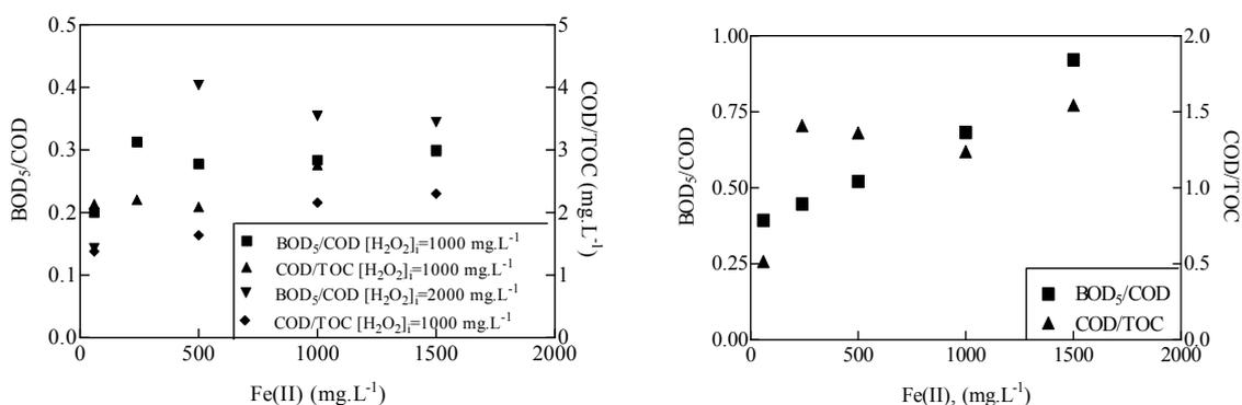
Figure 7.53: Evolution of the biodegradability and state of oxidation Vs. Fe(II) concentration at A) [H<sub>2</sub>O<sub>2</sub>]<sub>i</sub>=1000 and 2000 mg.L<sup>-1</sup>, B) [H<sub>2</sub>O<sub>2</sub>]<sub>i</sub>=1000 mg.L<sup>-1</sup> for photo-Fenton effluent solution, [POH]<sub>i</sub>=1000 mg.L<sup>-1</sup>, 15 min irradiation time and free pH evolutions.
