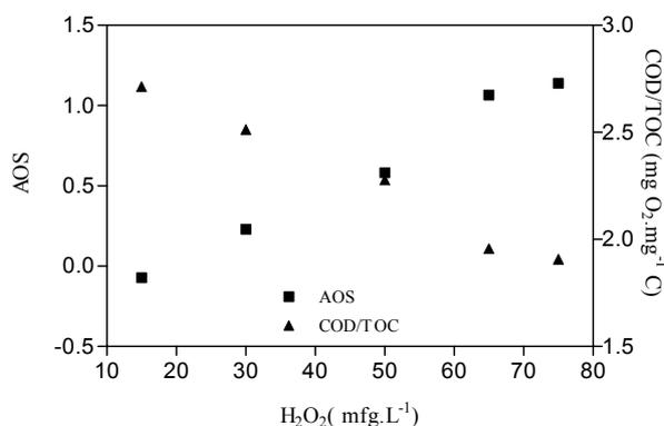
Figure 8.41: AOS and COD/TOC as function of initial  $H_2O_2$  in single lamp photo-reactor.  $[Fe(II)]_i = 10 \text{ mg.L}^{-1}$ , 50 min irradiation time and free pH evolution.
