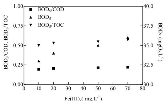
Figure 7.10: BOD<sub>5</sub>, BOD<sub>5</sub>/COD, BOD<sub>5</sub>/TOC evolution of POH treated solution as function of initial Fe(III) used in UV/Fe(III) process. Reaction time 90 min.
