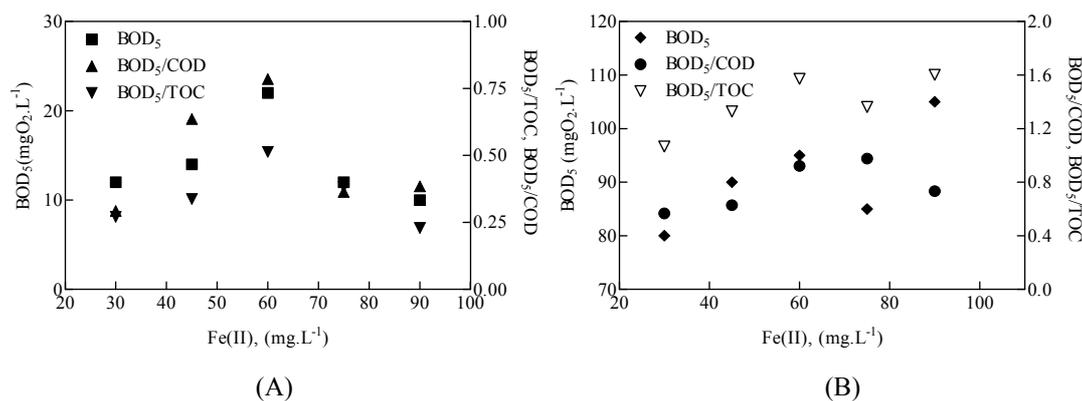
Figure 7.42: BOD<sub>5</sub>, BOD<sub>5</sub>/COD and BOD<sub>5</sub>/TOC as function of initial Fe (II) concentration for POH treated solution, A) [H<sub>2</sub>O<sub>2</sub>]<sub>i</sub>= 50 mg.L<sup>-1</sup>, 15 min reaction time and free pH evolution, B) [H<sub>2</sub>O<sub>2</sub>]<sub>i</sub>= 10 mg.L<sup>-1</sup>, 15 min reaction time and free pH evolution .
