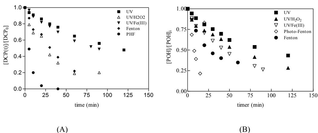
Figure 7.74. Comparison of the different processes for DCP and POH removal. A) DCP, [H<sub>2</sub>O<sub>2</sub>]<sub>i</sub> = 50 mg.L<sup>-1</sup>, [Fe(II)]<sub>i</sub> = 10 mg.L<sup>-1</sup>, [Fe(III)]<sub>i</sub> = 70 mg.L<sup>-1</sup> and free pH evolution, B) POH, [H<sub>2</sub>O<sub>2</sub>]<sub>i</sub> = 30 mg.L<sup>-1</sup>, [Fe(II)]<sub>i</sub> = 10 mg.L<sup>-1</sup>, [Fe(III)]<sub>i</sub> = 70 mg.L<sup>-1</sup> and free pH evolution
