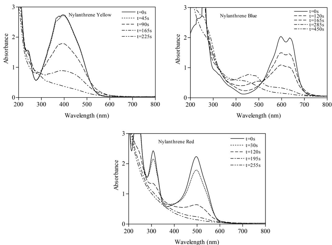
Figure 10.5 : VUV photolysis of Nylanthrene acid dyes ( $100 \text{ mg.L}^{-1}$ ).
