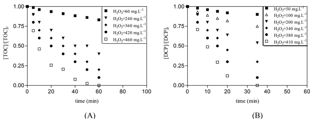
Figure 8.49: Normalized TOC evolution as function of time at different initial H<sub>2</sub>O<sub>2</sub> A) single lamp reactor B) multi lamps reactor. [Fe(II)]<sub>i</sub>= 10 mg.L<sup>-1</sup> and Free pH evolution
