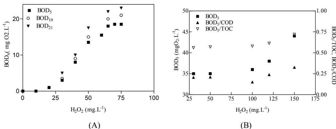
Figure 7.37:  $\text{BOD}_n$  as function of initial  $\text{H}_2\text{O}_2$  concentration for A) DCP Initial conditions, DCP are  $[\text{Fe}(\text{II})]_i = 10 \text{ mg}\cdot\text{L}^{-1}$ , 40 min reaction time and POH solution treated by photo-Fenton. and B) POH Initial conditions,  $[\text{Fe}(\text{II})]_i = 10 \text{ mg}\cdot\text{L}^{-1}$ , 15 min.
