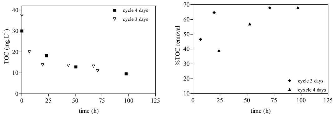
Figure 9.4: TOC evolution and organic matter removals (%TOC) as function of time for SBR operated at 4 and 3 days cycle duration , feed BOD<sub>5</sub>/COD= 0.25
