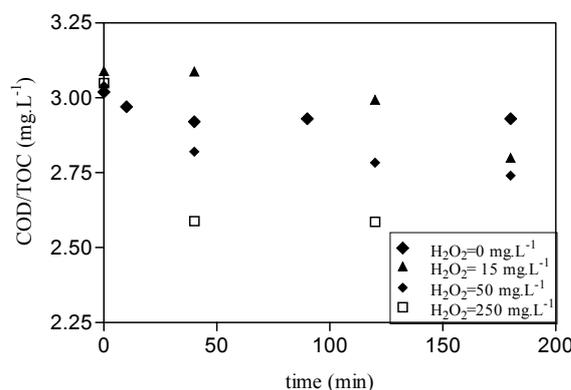
Figure 8.8: Evolution of COD/TOC vs. reaction time for UV/H<sub>2</sub>O<sub>2</sub> process at different initial H<sub>2</sub>O<sub>2</sub> concentrations in single lamp reactor.
