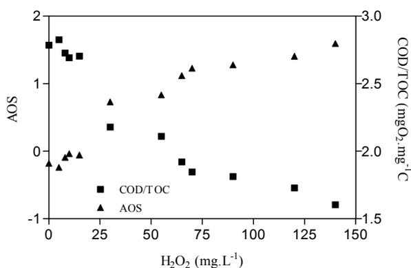
Figure 8.43: AOS and COD/TOC as function of initial  $H_2O_2$  in single lamp photo-reactor.  $[Fe(II)]_i = 10 \text{ mg.L}^{-1}$ , 35 min irradiation time and free pH evolution.
