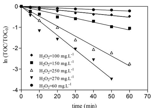
Figure 7.62: First order mineralization kinetics for DCP degradation.  $[Fe(II)]_i = 40$   $mg.L^{-1}$ , and free pH evolution.
