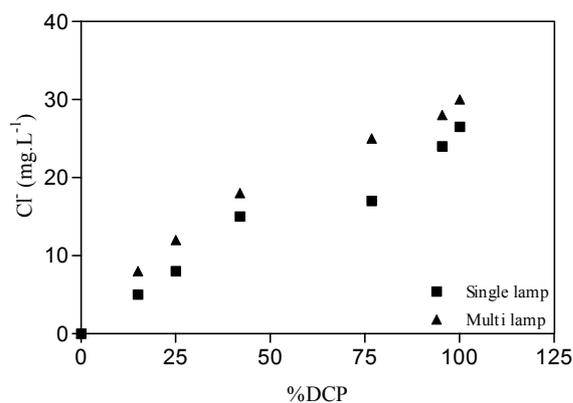
Figure 8.29: Dechlorination as function of DCP removal in single and multi lamps reactors.
