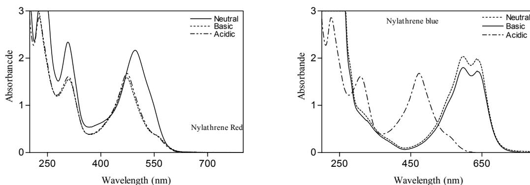
Figure 10.2: pH effect in UV-Vis. spectra for Nylathrene dyes
