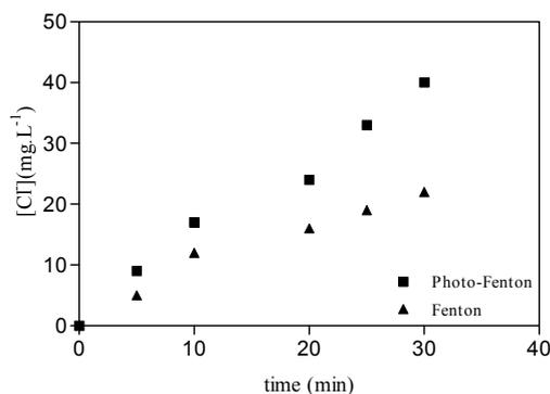
Figure 7.76: Dechlorination by Fenton and photo-Fenton process.  $[H_2O_2]_i = 50 \text{ mg.L}^{-1}$ ,  $[Fe(II)]_i = 10 \text{ mg.L}^{-1}$ ,  $[Fe(III)]_i = 70 \text{ mg.L}^{-1}$  and free pH evolution
