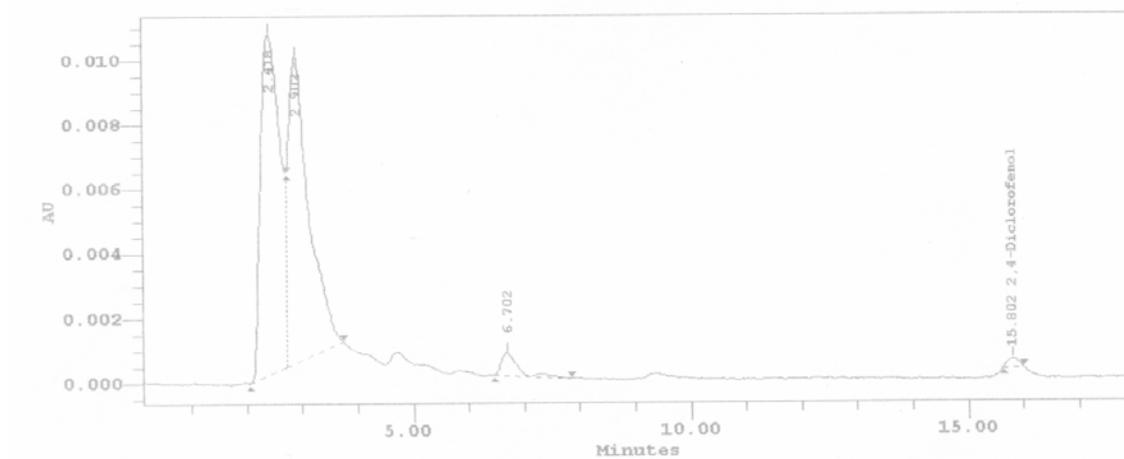
Figure A5.6: Chromatogram corresponding to sample at 30 min in photo-Fenton process
