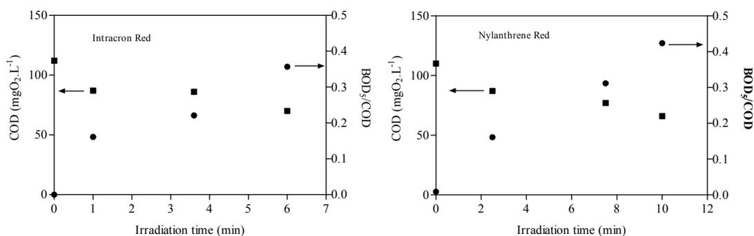
Figure 10.7: Evolution of  $\text{BOD}_5/\text{COD}$  ratio and COD vs irradiation time for Intracron Red and Nylanthrene Red ( $100 \text{ mg.L}^{-1}$ ).
