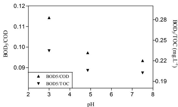
Figure 7.45: Change of BOD<sub>5</sub>/COD and BOD<sub>5</sub>/TOC as function of initial pH. [Fe (II)]<sub>i</sub>=10 mg.L<sup>-1</sup> and [H<sub>2</sub>O<sub>2</sub>]<sub>i</sub>= 30 mg.L<sup>-1</sup> and 40min experimental time
