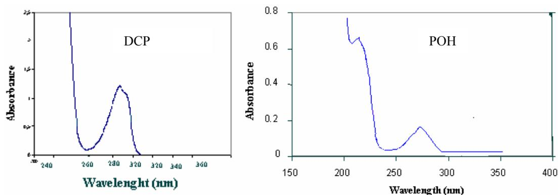
Figure 6.1 Absorption spectrum for DCP and POH
