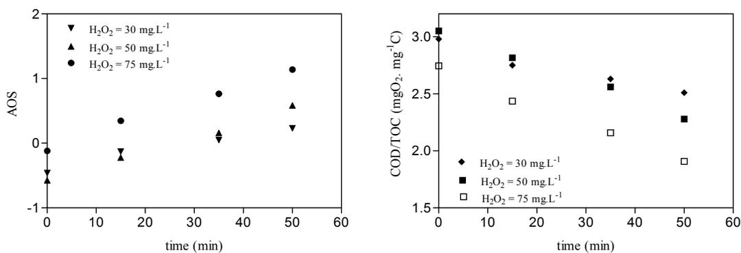
Figure 8.40: AOS and COD/TOC as function of time for different initial  $H_2O_2$  in single lamp photo-reactor.  $[Fe(II)]_i = 10 \text{ mg.L}^{-1}$ , 50 min irradiation time and free pH evolution.
