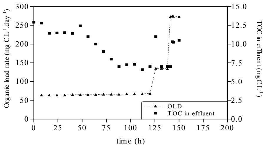
Figure 9.12 Evolution of total organic carbon (TOC) in effluent as function of operation hours.
