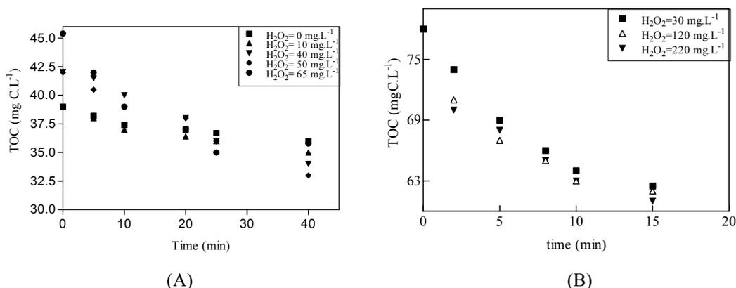
Figure 7.25: Total organic carbon evolution (TOC) in photo-Fenton reaction and different initial H<sub>2</sub>O<sub>2</sub> concentrations, A) DCP and B) POH. [Fe(II)]<sub>i</sub> = 10 mg. L<sup>-1</sup>, free pH evolution.
