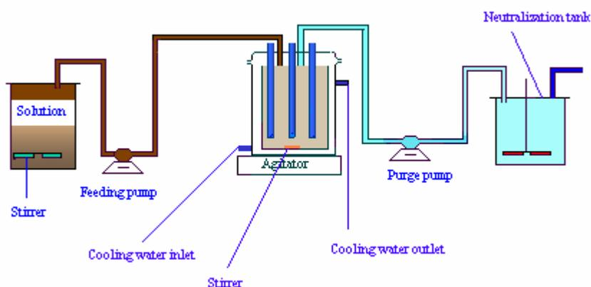
Figure 5.4: multi lamp stirred tank photo-reactors .
