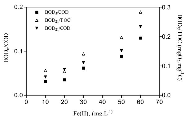
Figure 8.38: BOD<sub>n</sub>/COD and BOD<sub>5</sub>/TOC as function of initial Fe(II) in multi lamp photo-reactor. [H<sub>2</sub>O<sub>2</sub>]<sub>i</sub>= 15 mg.L<sup>-1</sup>, 35 min irradiation time and free pH evolution.
