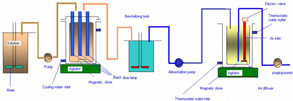
Figure 5.6: Photochemical-biological reactor installation
