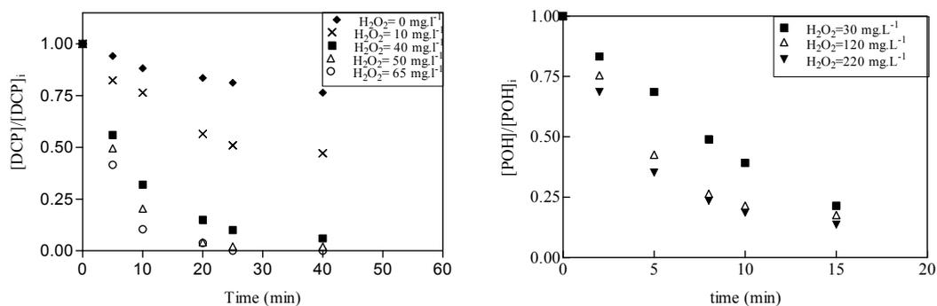
Figure 7.24: DCP and POH degradation in photo-Fenton reaction at different initial  $\text{H}_2\text{O}_2$  concentrations.  $[\text{Fe}(\text{II})]_i = 10 \text{ mg.L}^{-1}$ , free pH evolution.
