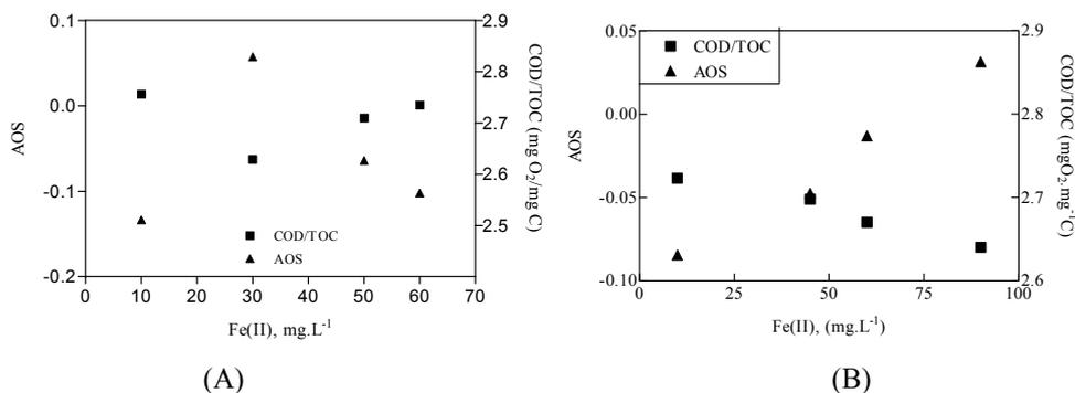
Figure 7.23: AOS and COD/TOC evolution of as a function of initial Fe (II) concentration for Fenton process. process (A) DCP [H<sub>2</sub>O<sub>2</sub>]<sub>i</sub> = 20 mg.L<sup>-1</sup>, 60 min reaction time and free pH evolution, (B) POH [H<sub>2</sub>O<sub>2</sub>]<sub>i</sub> = 30 mg.L<sup>-1</sup>, 30 min reaction time and free pH evolution,
