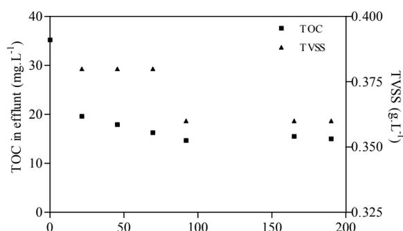
Figure 9.16: Evolution of organic matter and biomass concentration as function of cycle duration, cycle duration 8 days and feed  $\text{BOD}_5/\text{COD} = 0.15$ .
