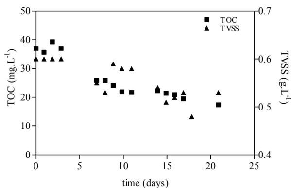
Figure 9.15: Total organic carbon (TOC) evolution and biomass concentration (TVSS) as function of acclimation time, feed BOD<sub>5</sub>/COD =0.15.
