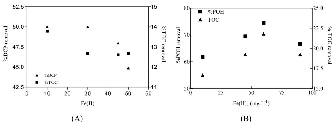
Figure 7.13: Evolution of DCP, POH and TOC removals as function of initial Fe (II) in Fenton process. (A)  $[\text{H}_2\text{O}_2]_i = 20 \text{ mg.L}^{-1}$ , 60 min reaction time and free pH evolution, (B) (A)  $[\text{H}_2\text{O}_2]_i = 30 \text{ mg.L}^{-1}$ , 30 min reaction time and free pH evolution.
