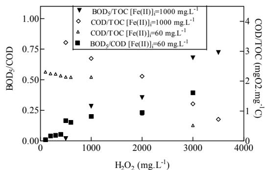
Figure 7.52: Evolution of the biodegradability and oxidation state Vs.  $\text{H}_2\text{O}_2$  concentration at  $[\text{Fe(II)}]_i=60 \text{ mg.L}^{-1}$  for photo-Fenton effluent solution,  $[\text{POH}]_i=1000 \text{ mg.L}^{-1}$ ,  $\text{pH}_0=3$
