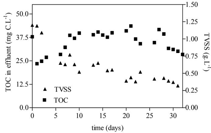
Figure 9.1: Total organic carbon evolution and TVSS as function of time during start up, feed BOD<sub>5</sub>/COD= 0.15
