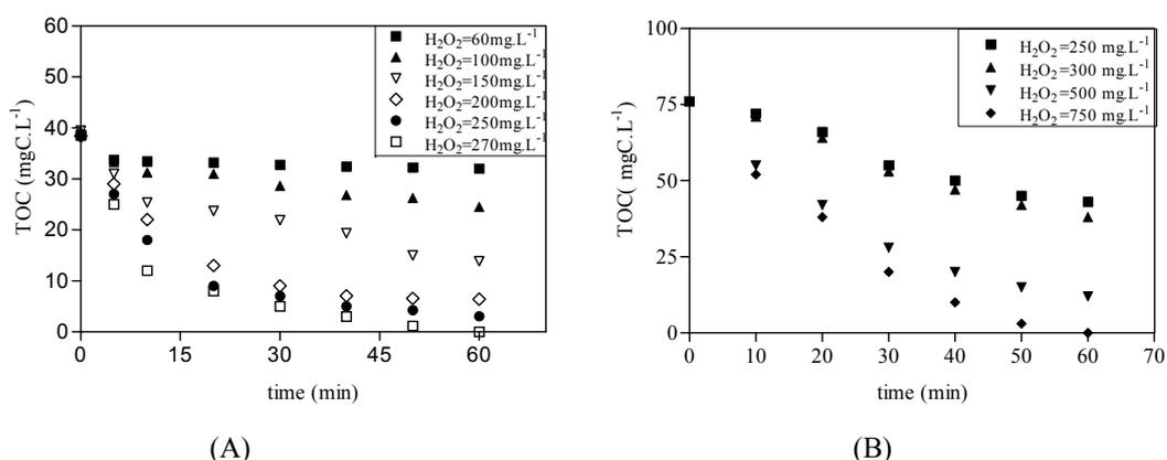
Figure 7.61: Mineralization of DCP and POH at different  $H_2O_2$  concentration, conditions A)  $[Fe(II)]_i=40$   $mg.L^{-1}$ , time=60 min and free pH evolution, B)  $[Fe(II)]_i=60$   $mg.L^{-1}$ , time=60 min and free pH evolution.
