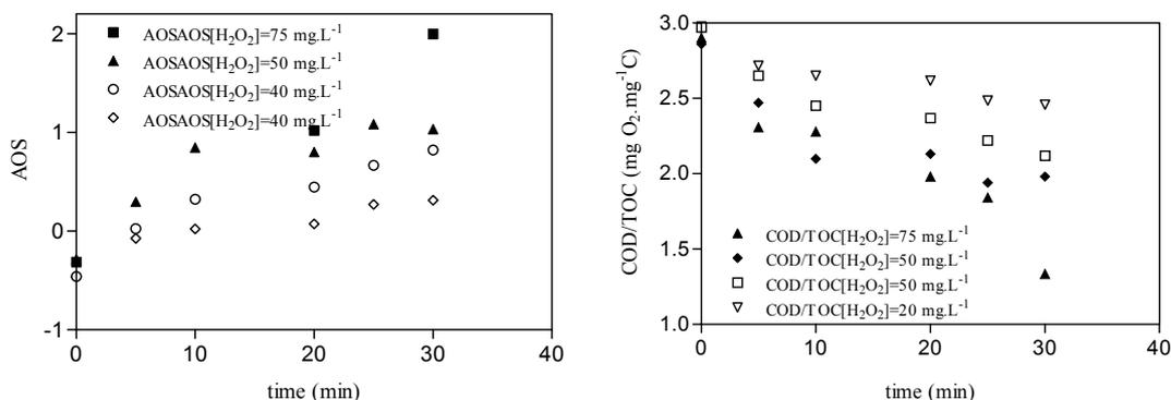
Figure 7.49: AOS and COD/TOC Evolution as reaction time for different initial  $H_2O_2$  Concentrations.  $[Fe(II)]_i = 10 \text{ mg.L}^{-1}$  and free pH evolutions
