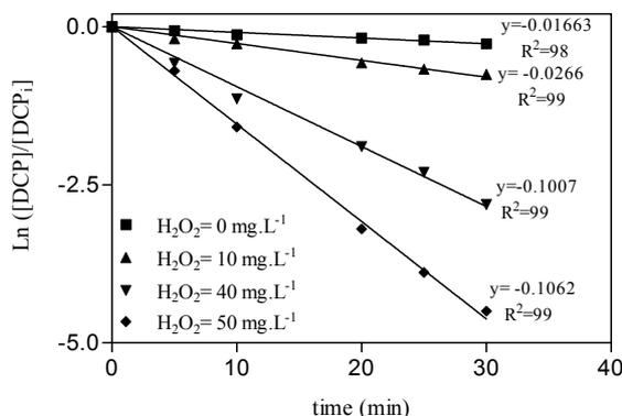
Figure 7.28: First-order plot for degradation of DCP as function of initial  $H_2O_2$ .  $[Fe(II)]_i=10 \text{ mg}\cdot\text{L}^{-1}$  and free pH evolution.
