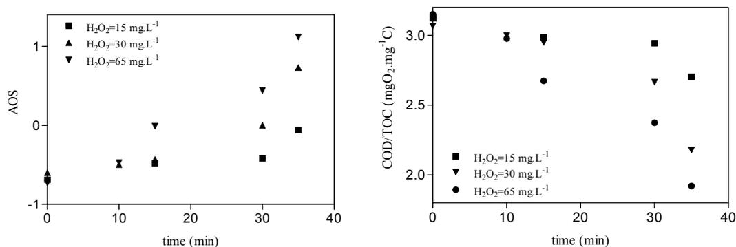
Figure 8.42: AOS and COD/TOC as function of time for different initial  $H_2O_2$  in multi lamps photo-reactor.  $[Fe(II)]_i = 10 \text{ mg.L}^{-1}$ , 35 min irradiation time and free pH evolution.
