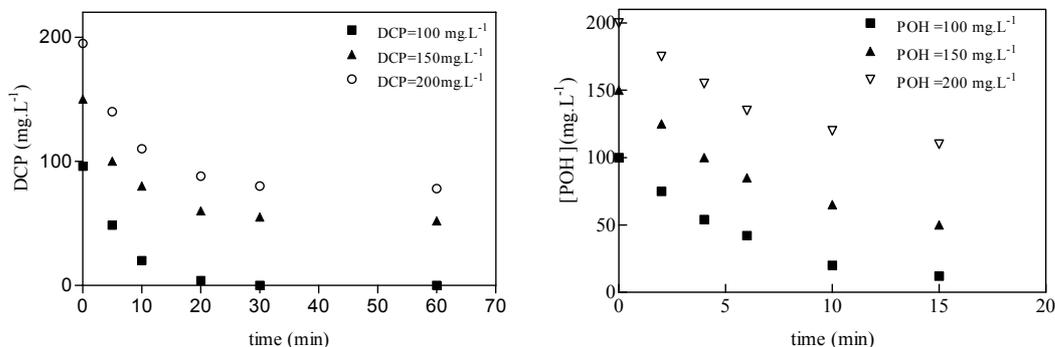
Figure 7.33: DCP and POH evolution as function of time for different initial concentrations, initial condition; for DCP are  $[H_2O_2]_i = 50 \text{ mg.L}^{-1}$   $[Fe(II)]_i = 10 \text{ mg.L}^{-1}$  and free pH evolution, for POH  $[H_2O_2]_i = 50 \text{ mg.L}^{-1}$   $[Fe(II)]_i = 60 \text{ mg.L}^{-1}$ .
