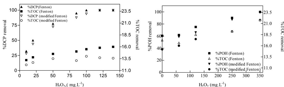
Figure 7.12: Evolution of DCP, POH and TOC removal in Fenton and modified Fenton as function of initial H<sub>2</sub>O<sub>2</sub>. [Fe (II)]<sub>i</sub> or [Fe (III)]<sub>i</sub> =10 mg.L<sup>-1</sup> and 60 min reaction time (30 min in POH case)
