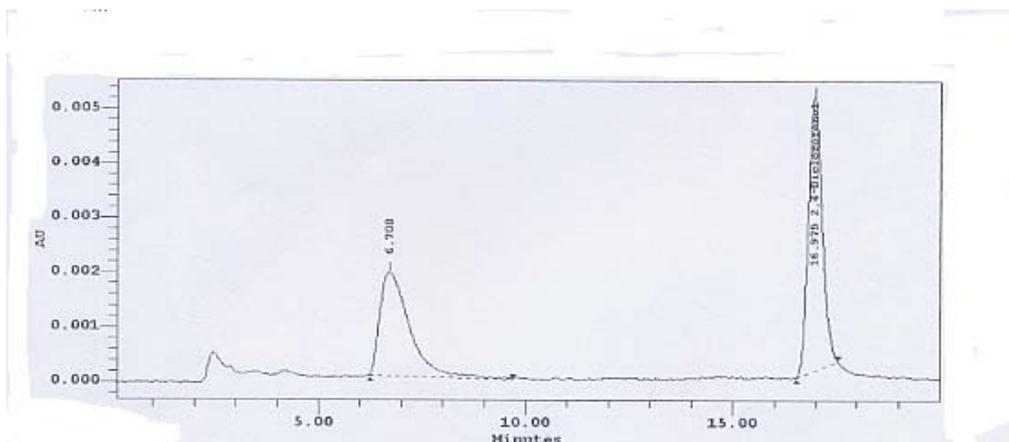
Figure 7.63: Chromatogram corresponding to sample at 30 min of direct UV-photolysis
