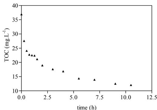
Figure 9.6: TOC evolution in aerobic SBR reactor during cycle of 12 h and feed  $BOD_5/COD=0.25$
