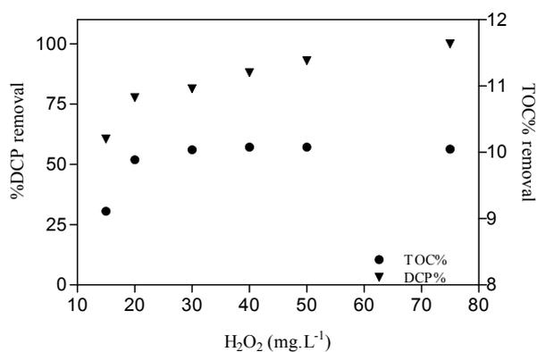
Figure 8.19: DCP removal as function of different initial  $H_2O_2$  concentration in single lamp photo-reactor  $[Fe(II)]_i = 10\text{ mg.L}^{-1}$  or
