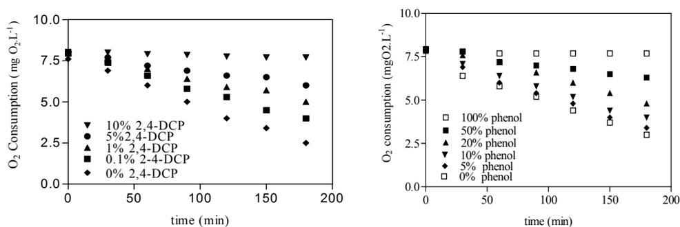
Figure 7.3: Inhibition test of oxygen consumption by activated sludge for 100 mg.L<sup>-1</sup> DCP and 100 mg.L<sup>-1</sup> POH solution.
