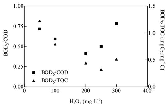
Figure: 7.39:  $BOD_5/COD$  and  $BOD_5/TOC$  as function of initial  $\text{H}_2\text{O}_2$  concentration for POH solution.  $[\text{Fe(II)}]_i = 60 \text{ mg}\cdot\text{L}^{-1}$ , 15 min reaction time.
