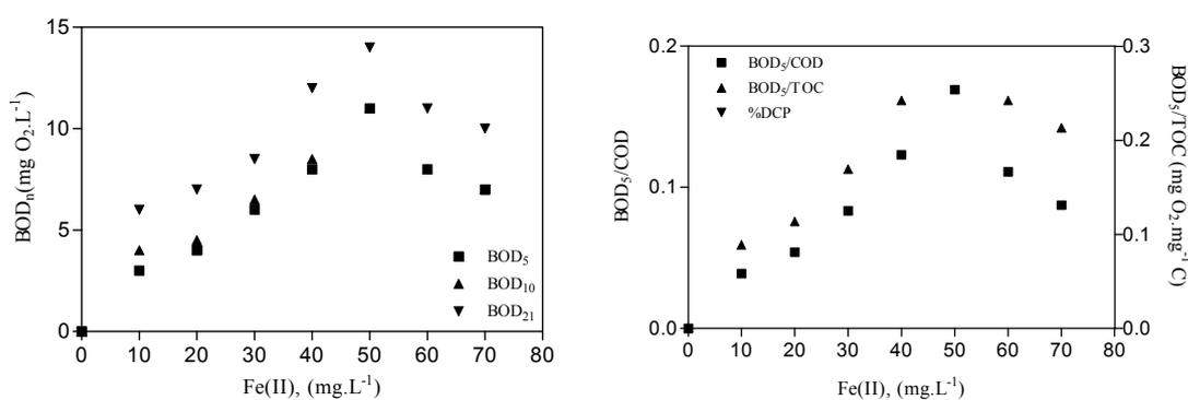
Figure 7.41:  $\text{BOD}_n$ ,  $\text{BOD}_5/\text{COD}$  and  $\text{BOD}_5/\text{TOC}$  as a function of initial Fe (II) concentration for DCP in photo-Fenton,  $[\text{H}_2\text{O}_2]_i = 30 \text{ mg}\cdot\text{L}^{-1}$ , 40 min reaction time.
