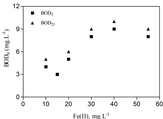
Figure 8.35 : BOD<sub>n</sub> as function of initial Fe(II) in single lamp photo-reactor. [H<sub>2</sub>O<sub>2</sub>]<sub>i</sub>= 30 mg.L<sup>-1</sup>, 50 min irradiation time and free pH evolution.
