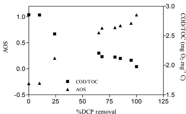
Figure 7.47: AOS and COD/TOC evolution as function of DCP removed.  $[Fe(II)]_i = 10 \text{ mg.L}^{-1}$ ,  $[H_2O_2]_i = 50$ , 40 min reaction time and free pH evolution .
