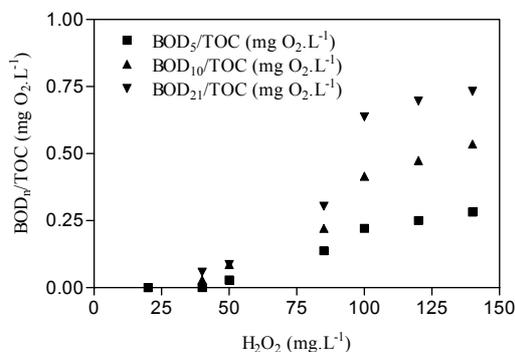
Figure 7.19: Change in BOD<sub>n</sub>/TOC ratios as function of initial H<sub>2</sub>O<sub>2</sub> concentration for DCP in Fenton and modified Fenton reactions. [Fe (II)]<sub>i</sub> or [Fe (III)]<sub>i</sub> = 10 mg.L<sup>-1</sup>, 60 min reaction time and free pH evolution.
