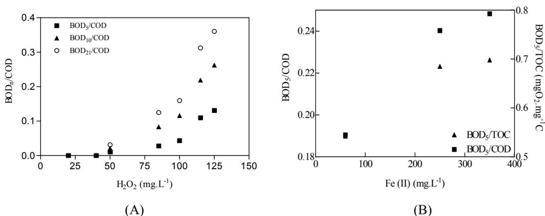
Figure 7.18: Change in BOD<sub>n</sub>/COD ratios as function of initial H<sub>2</sub>O<sub>2</sub> concentration for modified Fenton reaction. (A) DCP with [Fe(II)]<sub>i</sub> = 10 mg.L<sup>-1</sup>, 60 min reaction time ((30 min for POH) and free pH evolution, (B)POH with Fe(II)]<sub>i</sub> = 10 mg.L<sup>-1</sup>, 30 min reaction time and free pH evolution.
