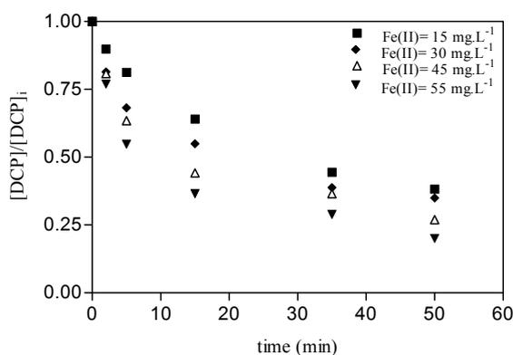
Figure 8.22: Evolution of normalized DCP concentration as function of time at different initial Fe(II) concentration in single lamp reactor.  $[\text{H}_2\text{O}_2]_i = 15 \text{ mg}\cdot\text{L}^{-1}$
