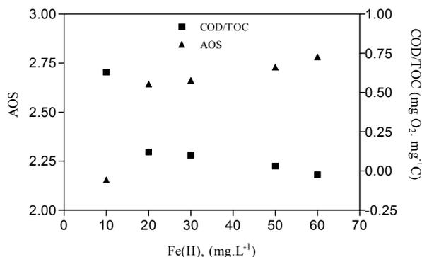
Figure 8.47: AOS and COD/TOC as function of initial Fe(II) in multi lamps photo-reactor.  $[H_2O_2]_i = 15 \text{ mg.L}^{-1}$ , 50 min irradiation time and free pH evolution.
