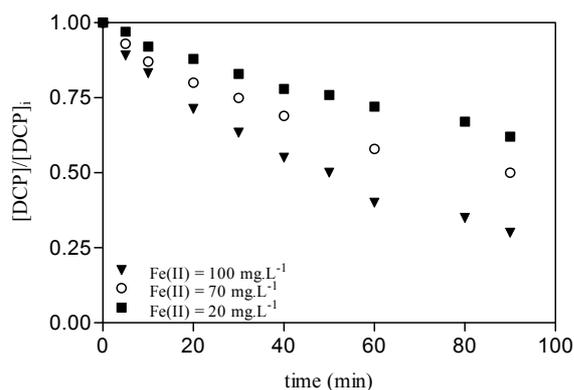
Figure 8.13 Evolution of DCP vs. reaction time at different initial Fe(III) concentrations in UVA/Fe(III) process in multi lamps reactor.
