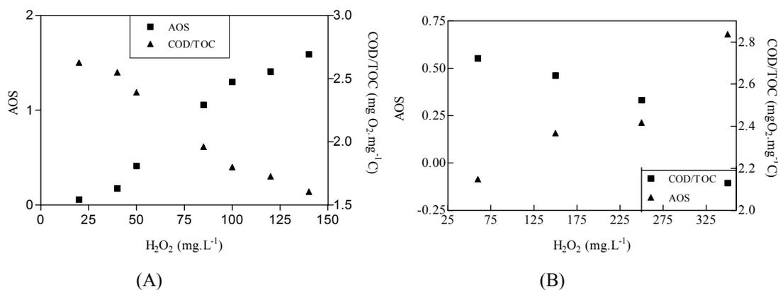
Figure 7.21: AOS and COD/TOC evolution of as a function of initial H<sub>2</sub>O<sub>2</sub> concentration for Fenton process. process (A) DCP [Fe (II)]<sub>i</sub> = 10 mg.L<sup>-1</sup>, 60 min reaction time and free pH evolution, (B) POH [Fe (II)]<sub>i</sub> = 10, 30 min reaction time and free pH evolution
