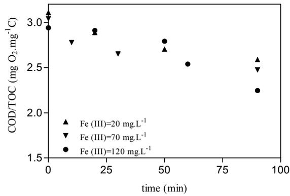
Figure 8.15: Evolution of COD/TOC as function of reaction time in UVA/Fe(III) process, for different initial Fe(III) concentrations in single lamp reactor.
