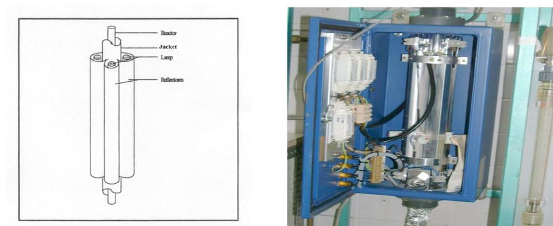
Figure (5.2) low-pressure mercury lamps and reflector configuration in photo-reactor
