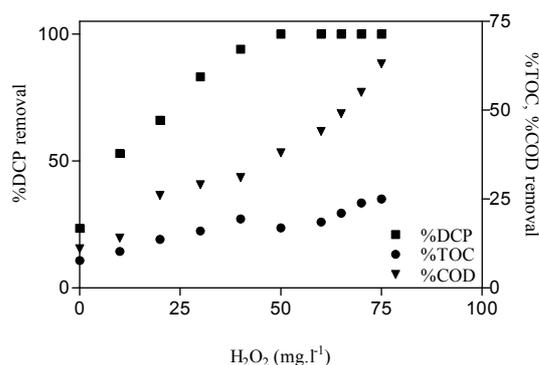
Figure 5.27: DCP, TOC and COD removal percentage as function of H<sub>2</sub>O<sub>2</sub> in photo-Fenton process. [Fe(II)]<sub>i</sub> = 10 mg. L<sup>-1</sup> experimental time 40 min.
