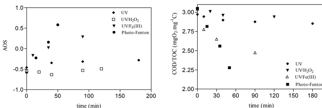
Figure 8.54: Change in oxidation state for the five AOP's, in single lamp photo-reactor.  $[H_2O_2]_i = 50 \text{ mg.L}^{-1}$ ,  $[Fe(III)]_i = 70 \text{ mg.L}^{-1}$ ,  $[Fe(II)]_i = 10 \text{ mg.L}^{-1}$ , and free pH evolutions.
