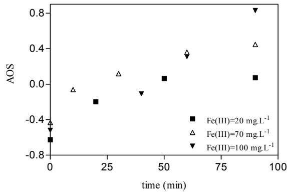
Figure 8.16: Evolution of AOS as function of reaction time in UVA/Fe(III) process, for different initial Fe(III) concentrations in multi lamps reactor.
