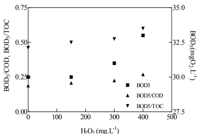
Figure 7.6: BOD<sub>5</sub>, BOD<sub>5</sub>/TOC and BOD<sub>5</sub>/COD Evolution of POH treated solution with UV/H<sub>2</sub>O<sub>2</sub> process
