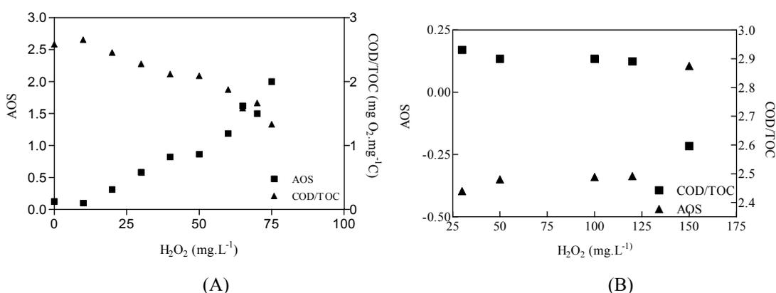
Figure 7.46: AOS and COD/TOC evolution as function of initial hydrogen peroxide (A) DCP.  $[Fe(II)]_i = 10 \text{ mg.L}^{-1}$ , 40 min reaction time and free pH evolution .B) (A) POH ,  $[Fe(II)]_i = 10 \text{ mg.L}^{-1}$ , 15 min reaction time and free pH evolution .
