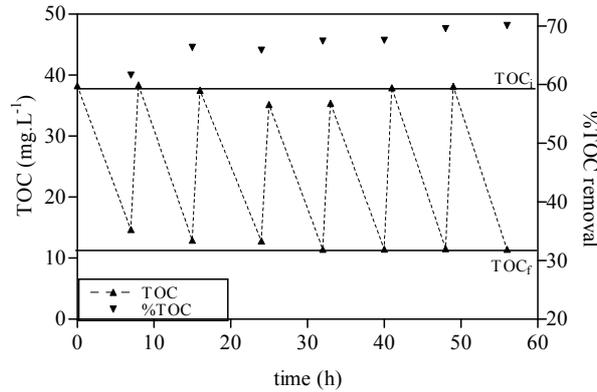
Figure 9.11: Evolution of initial organic carbon after feeding the reactor ( $TOC_i$ ), final organic carbon before next feeding ( $TOC_f$ ) and organic matter removal for each cycle (%TOC) as function of time, cycle duration 8 h and feed  $BOD_5/COD=0.35$ .
