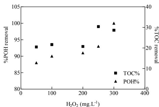
Figure 7.26: POH degradation in photo-Fenton reaction and different initial H<sub>2</sub>O<sub>2</sub> concentrations. [Fe(II)]<sub>i</sub> = 60 mg. L<sup>-1</sup>, free pH evolution, 15 min reaction time.
