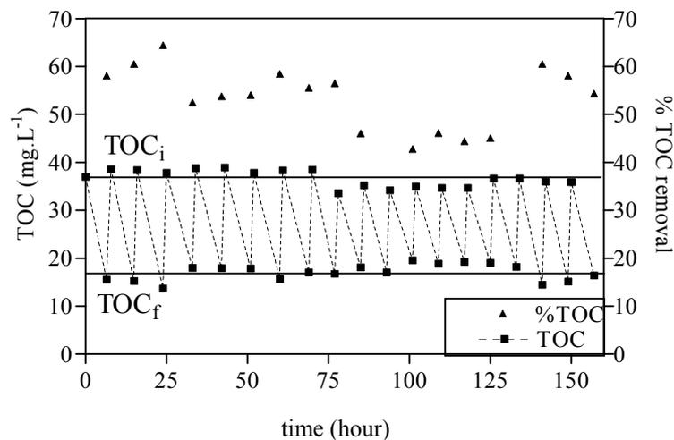
Figure 9.7: Evolution of initial organic carbon after feeding the reactor ( $TOC_i$ ), final organic carbon before next feeding ( $TOC_f$ ) and organic matter removal for each cycle (%TOC) as function of time, cycle duration 8 h and feed  $BOD_5/COD=0.25$ .
