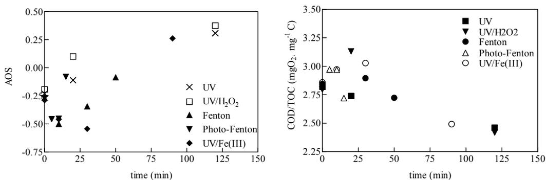
Figure 7.78: Change in oxidation state for the five processes during POH photo-degradation.  $[H_2O_2]_i = 30 \text{ mg}\cdot\text{L}^{-1}$ ,  $[Fe(II)]_i = 10 \text{ mg}\cdot\text{L}^{-1}$ ,  $[Fe(III)]_i = 70 \text{ mg}\cdot\text{L}^{-1}$  and free pH evolution.
