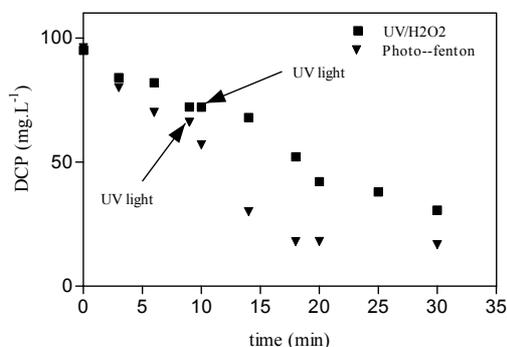
Figure 7.35: Variation of DCP as function of UV irradiation time for: UV/ $\text{H}_2\text{O}_2$  and photo-Fenton processes,  $[\text{H}_2\text{O}_2]_i = 30 \text{ mg}\cdot\text{L}^{-1}$ ,  $[\text{Fe}(\text{II})]_i = 10 \text{ mg}\cdot\text{L}^{-1}$
