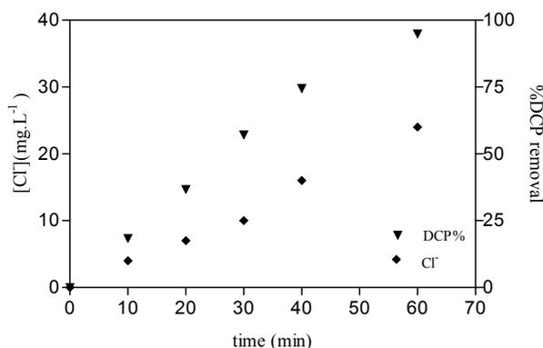
Figure 7.14: Evolution of chlorine ion and DCP removal as function of reaction time  $[\text{H}_2\text{O}_2]_i=85 \text{ mg.L}^{-1}$ ,  $[\text{Fe(II)}]_i=10 \text{ mg.L}^{-1}$  and free pH evolution.
