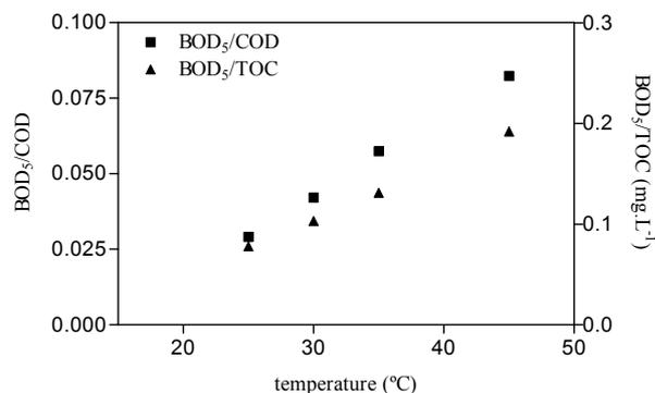
Figure 8.39: Variation of biodegradability as function of operational temperature in single lamp photo-reactor.  $[\text{H}_2\text{O}_2]_i = 30 \text{ mg.L}^{-1}$ ,  $[\text{Fe(II)}]_i = 10 \text{ mg.L}^{-1}$ , 50 min irradiation time and free pH evolution.
