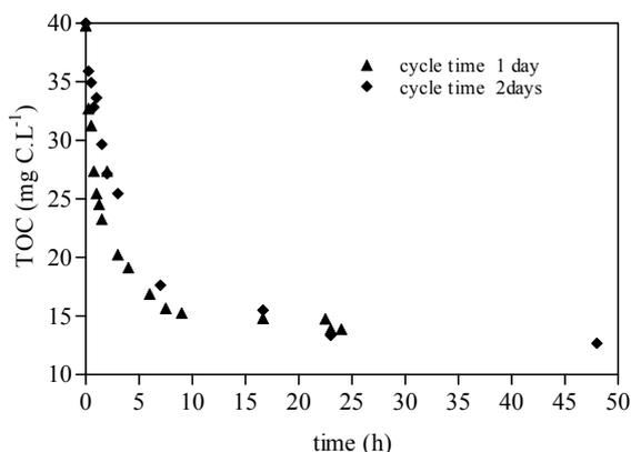
Figure 9.5: TOC evolution as function of time in aerobic SBR, cycle duration 1 and 2 days and feed  $BOD_5/COD=0.25$
