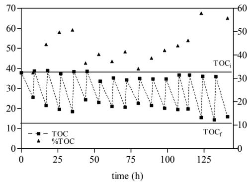
Figure 9.18: Evolution of initial organic carbon after feeding the reactor ( $TOC_i$ ), final organic carbon before next feeding ( $TOC_f$ ) and organic matter removal for each cycle ( $\%TOC$ ) as function of time, cycle duration 8h and feed  $BOD_5/COD=0.25$ .
