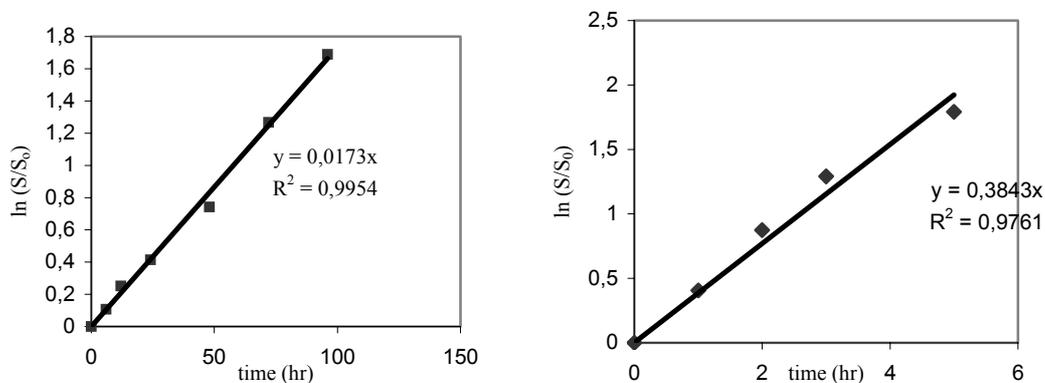
Figure 7.59: Kinetic study of aerobic biodegradation of A) POH, B) photo-Fenton effluent solution 100 mg.L<sup>-1</sup> POH, 50 mg.L<sup>-1</sup> H<sub>2</sub>O<sub>2</sub>, 75 mg.L<sup>-1</sup> Fe<sup>+2</sup>
