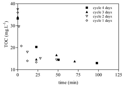
Figure 9.17: Evolution of organic matter as function of cycle duration, cycle duration 4,3, 2 and 1 day and feed  $BOD_5/COD = 0.25$ .
