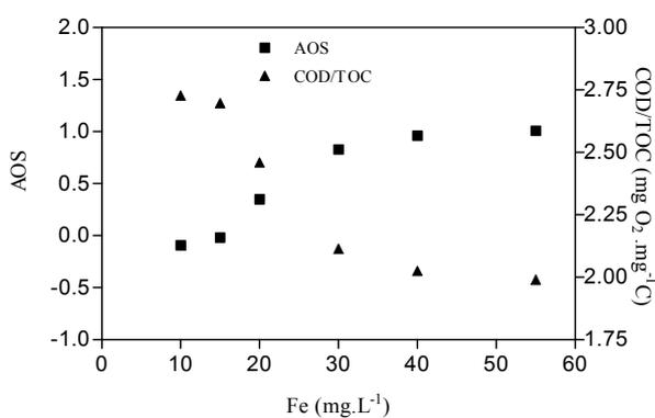
Figure 8.45: AOS and COD/TOC as function of initial Fe(II) in single lamp photo-reactor.  $[H_2O_2]_i = 30 \text{ mg.L}^{-1}$ , 50 min irradiation time and free pH evolution.
