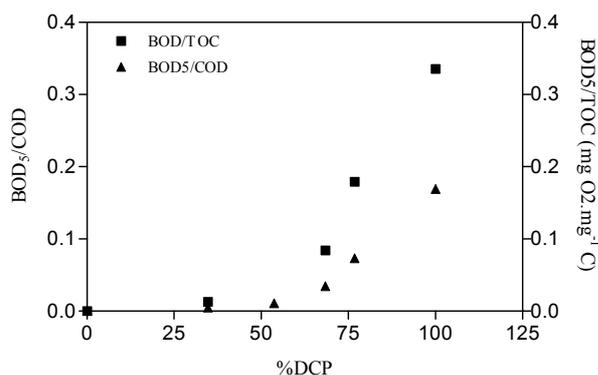
Figure 7.44: BOD<sub>5</sub>/COD and BOD<sub>5</sub>/TOC change as a function DCP removal, [Fe (II)]<sub>i</sub>= 30 mg. L<sup>-1</sup> and [H<sub>2</sub> O<sub>2</sub>]<sub>i</sub>= 30 mg. L<sup>-1</sup> for 40 min and free pH evolution.
