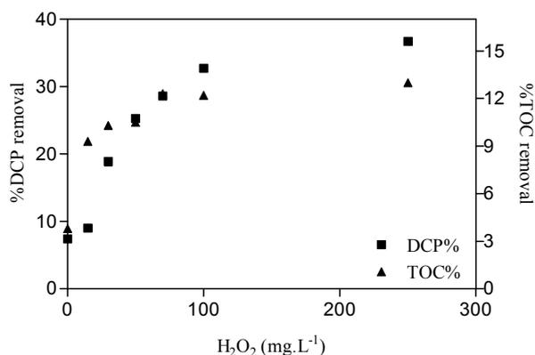
Figure 8.2: DCP and TOC removal percentage as function of  $H_2O_2$  in UVA/ $H_2O_2$  process for single lamp reactor, irradiation time 2 hours.
