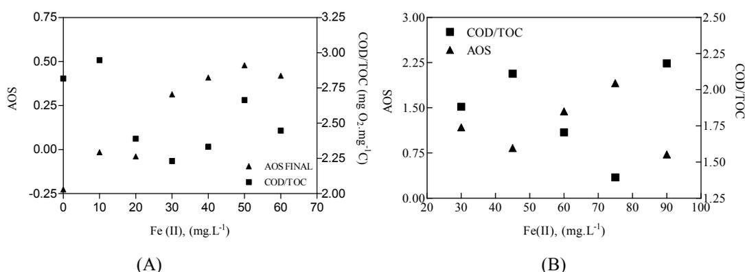
Figure 7.48: AOS and COD/TOC as function of initial Fe(II). Initial conditions, A) DCP  $[\text{H}_2\text{O}_2]_i = 10 \text{ mg}\cdot\text{L}^{-1}$ , 40 min reaction time and B) POH  $[\text{H}_2\text{O}_2]_i = 50 \text{ mg}\cdot\text{L}^{-1}$ , 15 min reaction time.
