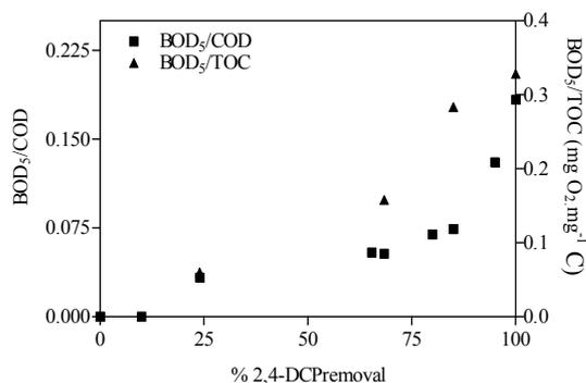
Figure 7.40:  $BOD_5/COD$  and  $BOD_5/TOC$  as a function DCP removal percentage.  $[\text{H}_2\text{O}_2]_i = 50 \text{ mg}\cdot\text{L}^{-1}$ ,  $[\text{Fe(II)}]_i = 10 \text{ mg}\cdot\text{L}^{-1}$  40 min and free pH evolution.
