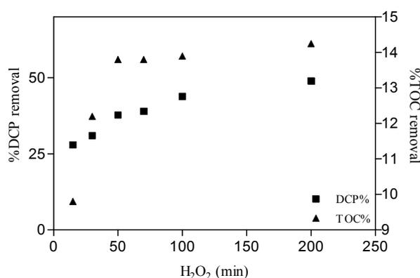
Figure 8.4: DCP and TOC removal percentage as function of  $\text{H}_2\text{O}_2$  in UVA/ $\text{H}_2\text{O}_2$  process for multi lamps reactor, irradiation time 2 hours.
