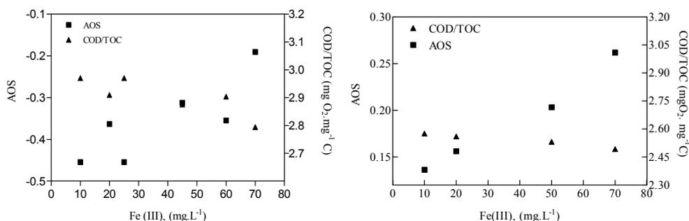
Figure 7.11: Evolution of COD/TOC and AOS as a function of initial Fe (III) concentration for DCP and POH in UV/Fe (III) process. Reaction time 90 min.
