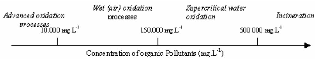
Figure 3-1: Suitability of water treatment technologies according to COD contents (Andreozzi et al., 1999)
