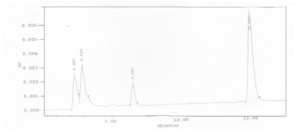
Figure A5.1: Chromatogram corresponding to sample at 20 min in UVA/H<sub>2</sub>O<sub>2</sub> process
