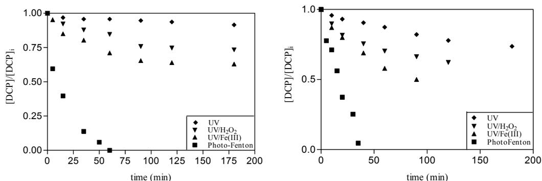
Figure 8.50: DCP evolution as function of time for different AOP's in single and multi lamps reactor.  $[H_2O_2]_i = 50 \text{ mg.L}^{-1}$ ,  $[Fe(III)]_i = 70 \text{ mg.L}^{-1}$ ,  $[Fe(II)]_i = 10 \text{ mg.L}^{-1}$  and free ph evolution.
