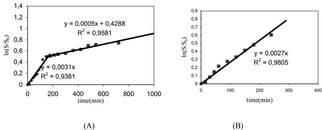
Figure 7.57: Kinetic study of the biodegradation of 100% pre-treated solution carried out in the acclimated reactor. Conditions: (A) T = 22°C, pH ≈ 7.2, TVSS = 0.13 g.L<sup>-1</sup>, HRT = 1 days, (B) (A) T = 22°C, pH ≈ 7.2, TVSS = 0.13 g.L<sup>-1</sup>, HRT = 12 h
