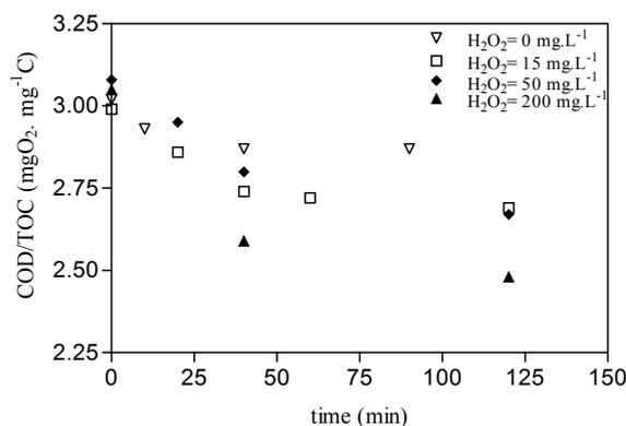
Figure 8.10: Evolution of COD/TOC vs. reaction time for UVA/H<sub>2</sub>O<sub>2</sub> process at different initial H<sub>2</sub>O<sub>2</sub> concentrations in multi lamps reactor.
