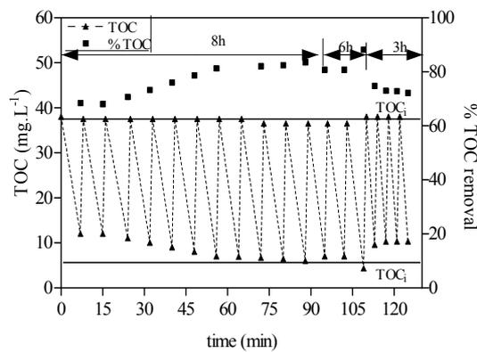
Figure 9.12: Evolution of initial organic carbon after feeding the reactor ( $TOC_i$ ), final organic carbon before next feeding ( $TOC_f$ ) and organic matter removal for each cycle ( $\%TOC$ ) as function of time, cycle duration 8 h and feed  $BOD_5/COD= 0.48$ .
