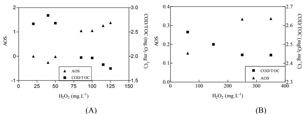
Figure 7.22: AOS and COD/TOC evolution of as a function of initial H<sub>2</sub>O<sub>2</sub> concentration for modified Fenton process (A) DCP [Fe (II)]<sub>i</sub> = 10 mg.L<sup>-1</sup>, 60 min reaction time and free pH evolution, (B) POH [Fe (II)]<sub>i</sub> = 10, 30 min reaction time and free pH evolution
