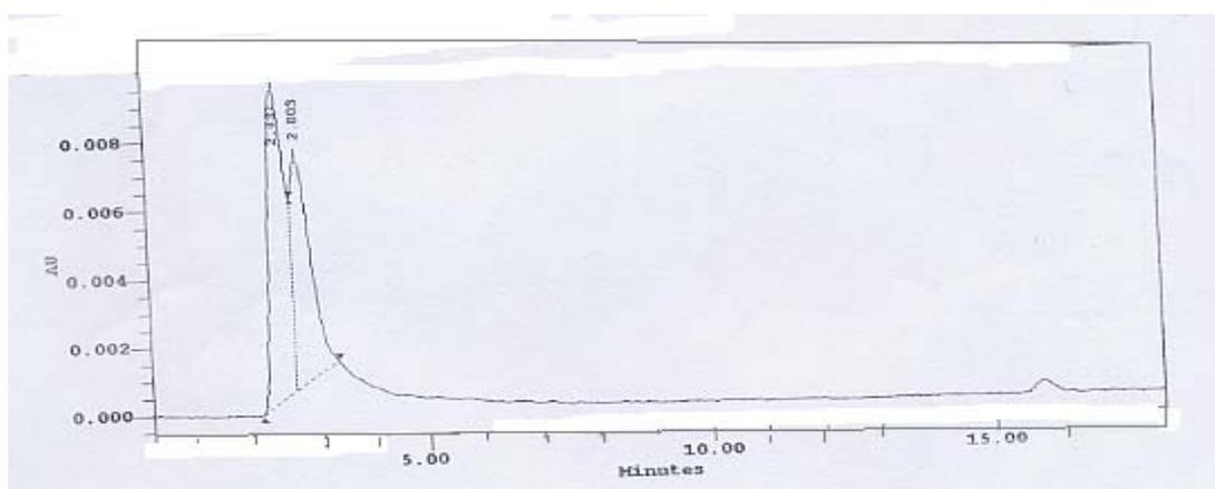
Figure 7.72: Chromatogram corresponding to sample at 5.0 min of photo-Fenton reaction
