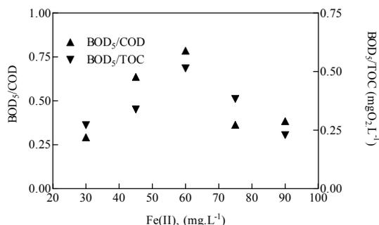
Figure 7.43: BOD<sub>5</sub>/COD and BOD<sub>5</sub>/TOC as function of initial Fe (II) concentration for photo-Fenton, [H<sub>2</sub>O<sub>2</sub>]<sub>i</sub>= 300 mg·L<sup>-1</sup>, 40 min reaction time.
