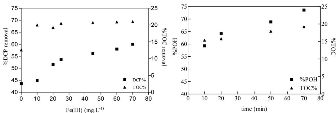
Figure 7.8: Evolution of DCP, POH and TOC as function of initial Fe (III) concentration during UV/ Fe (III) process. Reaction time 90 min
