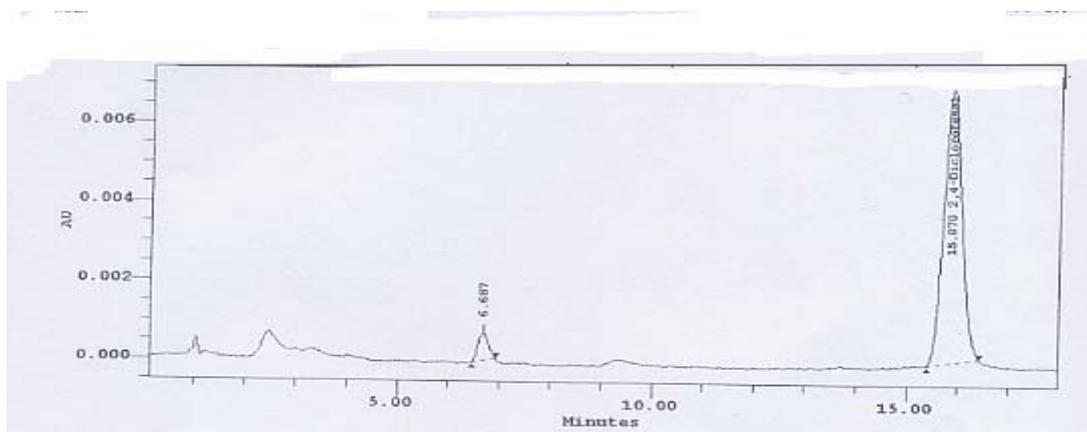
Figure 7.70: Chromatogram corresponding to sample at 0.5 min of photo-Fenton reaction
