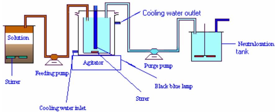
Figure 5.3; Single lamp stirred tank photo-reactors .
