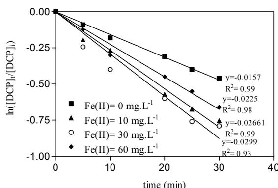
Figure 7.31: First-order plot for degradation of DCP as function of initial Fe (II) in photo-Fenton reaction:  $[\text{H}_2\text{O}_2]_0 = 10 \text{ mg.L}^{-1}$  and free pH evolutions.
