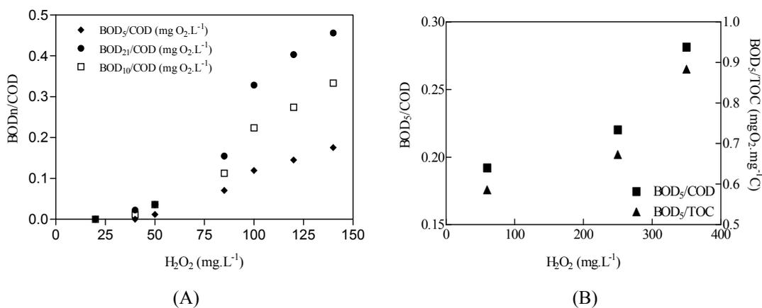
Figure 7.17: Change in Bon<sub>n</sub>/COD ratios as function of initial H<sub>2</sub>O<sub>2</sub> concentration in Fenton reaction. (A) DCP with [Fe(II)]<sub>i</sub> = 10 mg.L<sup>-1</sup>, 60 min reaction time ((30 min for POH) and free pH evolution, (B)POH with Fe(II)]<sub>i</sub> = 10 mg.L<sup>-1</sup>, 30 min reaction time and free pH evolution.
