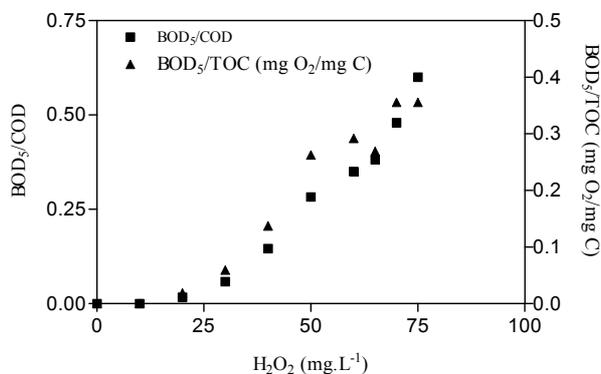
Figure 7.38: BOD<sub>5</sub>/COD and BOD<sub>5</sub>/TOC as function of initial H<sub>2</sub>O<sub>2</sub> concentration for DCP solution. [Fe (II)]<sub>i</sub>= 10 mg-L<sup>-1</sup>, 40 min reaction time.
