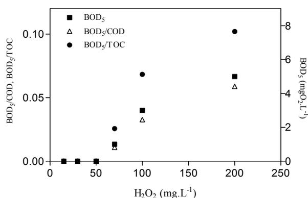
Figure 8.6:  $BOD_5$ ,  $BOD_5/COD$  and  $BOD_5/TOC$  as function of initial  $H_2O_2$  in UVA/ $H_2O_2$  for multi lamps reactor, reaction time 90 min.
