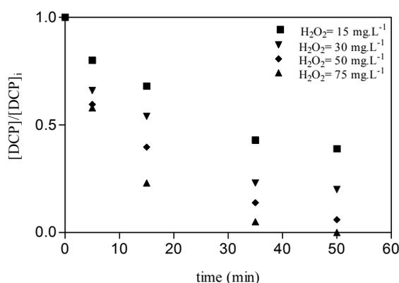
Figure 8.18. Evolution of DCP as function of irradiation time at different  $H_2O_2$  in single lamp photo-reactor  $[Fe(II)]_i = 10\text{ mg.L}^{-1}$
