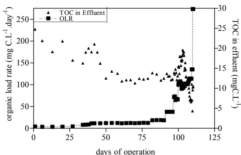
Figure 9.2: TOC in effluent solution as function of operation days for aerobic SBR. Feed BOD<sub>5</sub>/COD=0.25.
