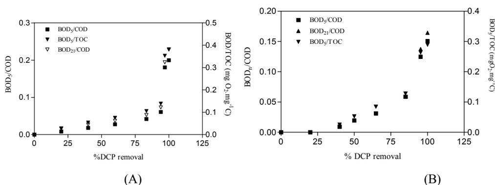
Figure 8.34: BOD<sub>5</sub>/COD and BOD<sub>5</sub>/TOC as a function DCP removal percentage A) single lamp reactor with [H<sub>2</sub>O<sub>2</sub>]<sub>i</sub>= 75 mg.L<sup>-1</sup>, [Fe(II)]<sub>i</sub>=10 mg.L<sup>-1</sup> 50 min and free pH evolution, B) multi lamps reactor with [H<sub>2</sub>O<sub>2</sub>]<sub>i</sub>= 65 mg.L<sup>-1</sup>, [Fe(II)]<sub>i</sub>=10 mg.L<sup>-1</sup> 35 min and free pH evolution.
