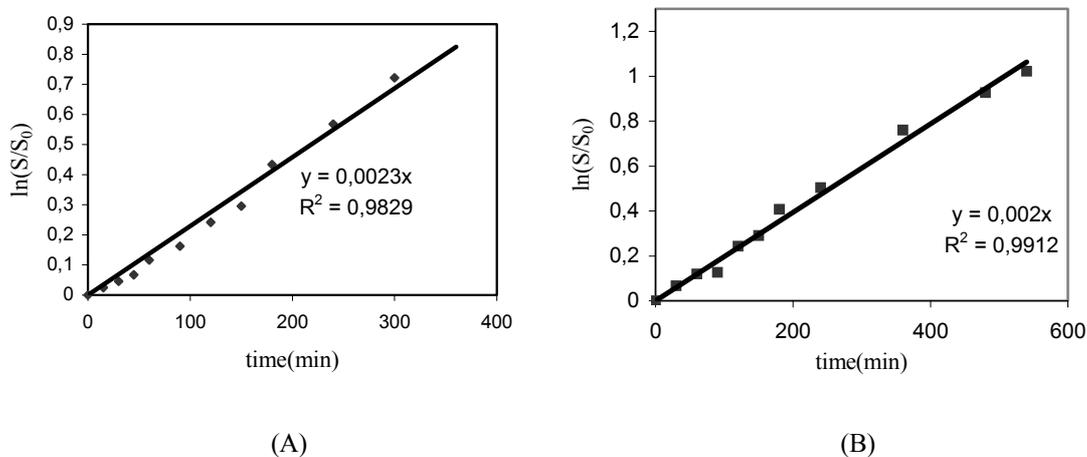
Figure 7.55. Kinetic study of the biodegradation of 100% pre-treated solution carried out in the non-acclimated reactor. Conditions:  $T = 22^\circ\text{C}$ ,  $\text{pH} \approx 7.2$ ,  $\text{TVSS} = 0.35 \text{ g} \cdot \text{L}^{-1}$ , (A)  $\text{HRT} = 2$  days and (B)  $T = 22^\circ\text{C}$ ,  $\text{pH} \approx 7.2$ ,  $\text{TVSS} = 0.35 \text{ g} \cdot \text{L}^{-1}$   $\text{HRT} = 1$  days.
