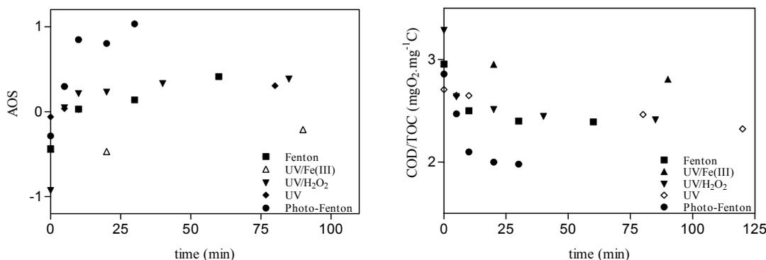
Figure 7.77: Change in oxidation state for the five processes during DCP photo-degradation.  $[H_2O_2]_i = 50 \text{ mg.L}^{-1}$ ,  $[Fe(II)]_i = 10 \text{ mg.L}^{-1}$ ,  $[Fe(III)]_i = 70 \text{ mg.L}^{-1}$  and free pH evolution.
