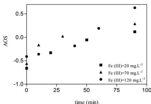
Figure 8.14: Evolution of AOS as function of reaction time in UVA/ $\text{Fe(III)}$  process, for different initial  $\text{Fe(III)}$  concentrations in single lamp reactor.
