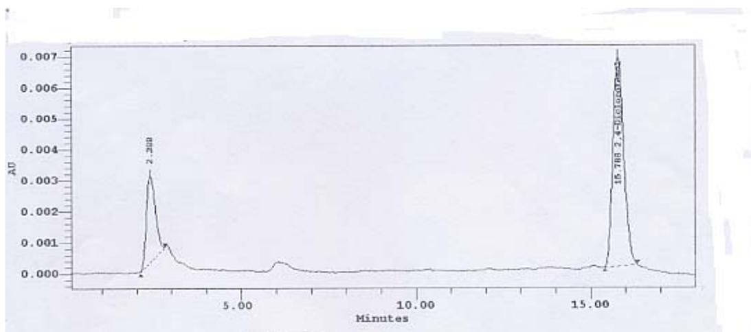
Figure 7.71: Chromatogram corresponding to sample at 1.0 min of photo-Fenton reaction
