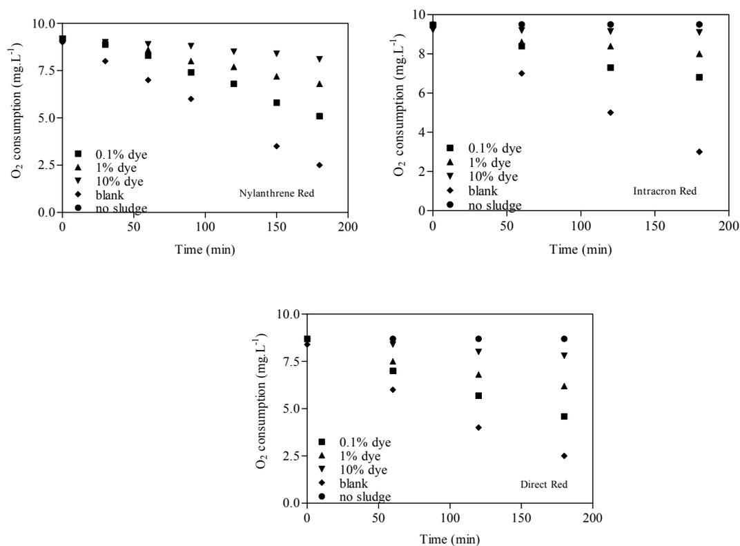
Figure 10.4 : Inhibition of O<sub>2</sub> consumption by activated sludge for three dye solutions (100mg.L<sup>-1</sup>, pH= 7.0± 0.2 )
