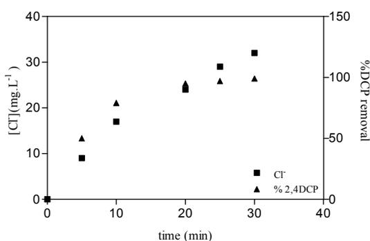
Figure 7.36: Evolution of chloride ion and DCP % elimination as function of reaction time.  $[\text{H}_2\text{O}_2]=50 \text{ mg.L}^{-1}$ ,  $[\text{Fe}(\text{II})]=10 \text{ mg.L}^{-1}$ .
