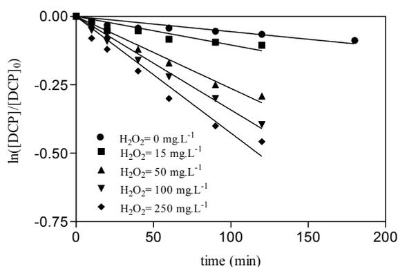
Figure 8.5: First order kinetics for DCP degradation by UVA/ $\text{H}_2\text{O}_2$  process. At different  $\text{H}_2\text{O}_2$  initial concentration in single lamp reactor
