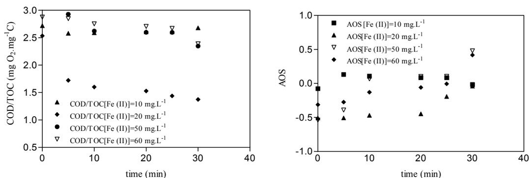
Figure 7.50: AOS and COD/TOC Evolution as reaction time for different initial Fe (II) Concentrations.  $[H_2O_2]_i = 10 \text{ mg.L}^{-1}$  and free pH evolutions
