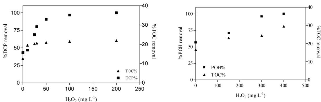
Figure 7.4: DCP, POH and TOC removal as function of initial  $H_2O_2$  concentration during UV/  $H_2O_2$  process. Reaction time 90 min .
