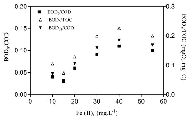
Figure 8.37 : BOD<sub>n</sub>/COD and BOD<sub>5</sub>/TOC as function of initial Fe(II) in single lamp photo-reactor. [H<sub>2</sub>O<sub>2</sub>]<sub>i</sub>= 30 mg.L<sup>-1</sup>, 50 min irradiation time and free pH evolution.
