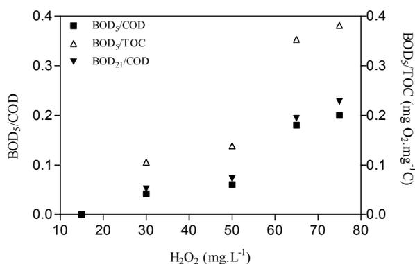
Figure 8.32: Evolution of  $\text{BOD}_n/\text{COD}$  and  $\text{BOD}_n/\text{TOC}$  as function of initial  $\text{H}_2\text{O}_2$  in single lamp photo-reactor.  $[\text{Fe(II)}]_i = 10 \text{ mg.L}^{-1}$ , 50 min irradiation time and free pH evolution.
