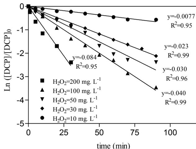
Figure 7.5: First order kinetic constant for DCP degradation by UV/ $H_2O_2$  photolysis
