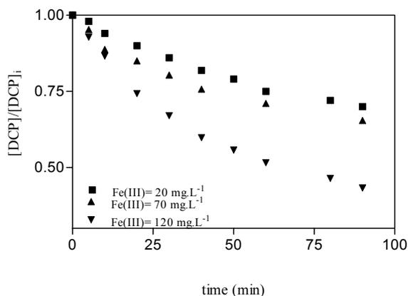
Figure 8.11 Evolution of DCP vs. reaction time at different initial Fe(III) concentrations in UVA/Fe(III) process in single lamp reactor.
