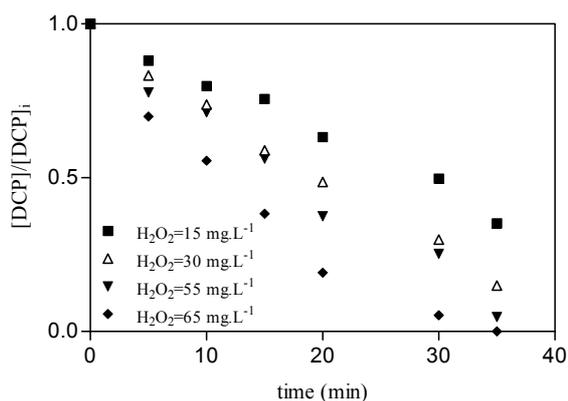
Figure 8.20. Evolution of DCP as function of irradiation time at different  $\text{H}_2\text{O}_2$  in multi lamps photo-reactor.  $[\text{Fe(II)}]_i = 10 \text{ mg. L}^{-1}$
