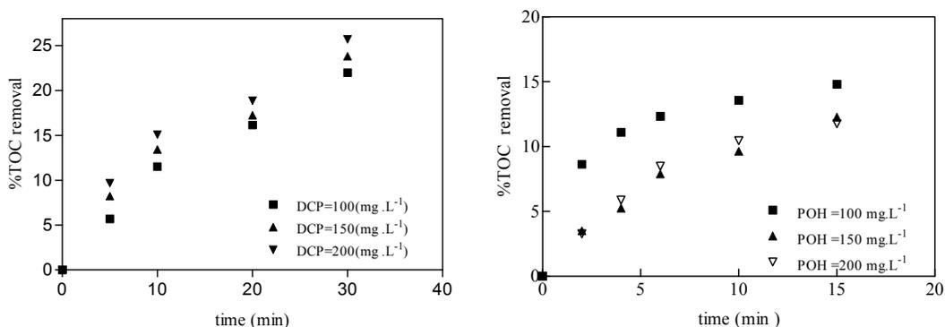
Figure 7.34: Evolution of TOC vs. reaction time for different DCP and POH initial concentrations, initial condition; for DCP are  $[H_2O_2]_i = 50 \text{ mg.L}^{-1}$   $[Fe(II)]_i = 10 \text{ mg.L}^{-1}$  and free pH evolution, for POH  $[H_2O_2]_i = 50 \text{ mg.L}^{-1}$   $[Fe(II)]_i = 60 \text{ mg.L}^{-1}$ .
