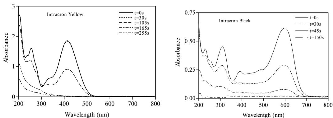
Figure 10.6 : UV Photolysis of Intracron reactive dyes ( $100 \text{ mg.L}^{-1}$ ).
