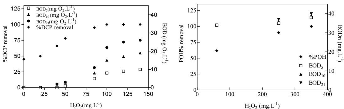
Figure 7.15: Evolution of  $\text{BOD}_n$ , DCP removal and POH removal as function of initial  $\text{H}_2\text{O}_2$  in Fenton reaction.  $[\text{Fe}(\text{II})]_i = 10$ , 60 min reaction time (30 min for POH) and free pH evolution.
