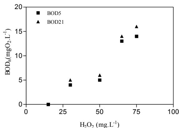
Figure 8.30: Evolution of  $\text{BOD}_n$  as function of initial  $\text{H}_2\text{O}_2$  in single lamp photo-reactor.  $[\text{Fe(II)}]_i = 10 \text{ mg}\cdot\text{L}^{-1}$ , 50 min irradiation time and free pH evolution.
