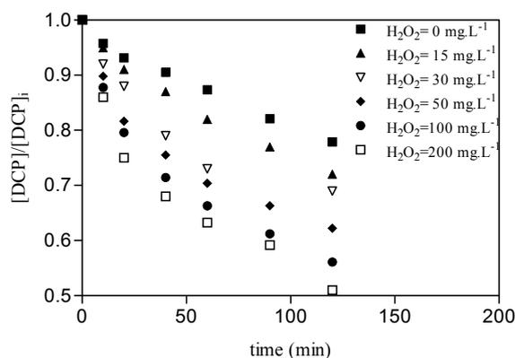
Figure 8.3: Evolution of DCP vs. reaction time for different  $\text{H}_2\text{O}_2$  initial concentration in UVA/ $\text{H}_2\text{O}_2$  process for multi lamps reactor.
