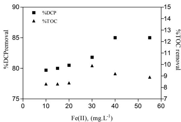
Figure 8.24: DCP and TOC degradation as function of iron catalyst in photo-Fenton process in single lamp reactor.  $[H_2O_2]_i = 30 \text{ mg.L}^{-1}$  and 50 min irradiation.
