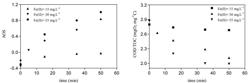
Figure 8.44: AOS and COD/TOC as function of time at different initial Fe(II) in single lamp photo-reactor.  $[H_2O_2]_i = 30 \text{ mg.L}^{-1}$ , 50 min irradiation time and free pH evolution.
