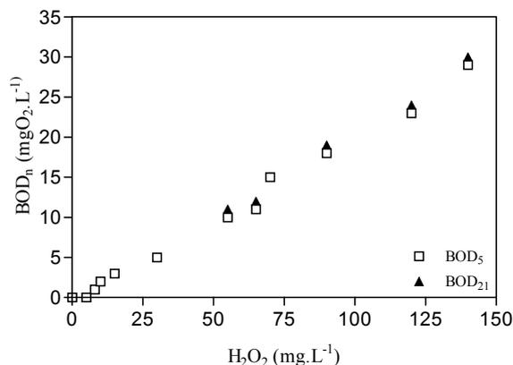
Figure 8.31: Evolution of  $\text{BOD}_n$  as function of initial  $\text{H}_2\text{O}_2$  in multi lamps photo-reactor.  $[\text{Fe(II)}]_i = 10 \text{ mg.L}^{-1}$ , 35 min irradiation time and free pH evolution.
