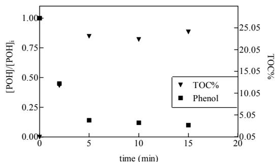
Figure 7.51: Variation of POH concentration and TOC removal percentage COD/TOC and ratio for photo-Fenton effluent solution ( $1000 \text{ mg.L}^{-1}$  POH,  $3000 \text{ mg.L}^{-1}$   $\text{H}_2\text{O}_2$  and  $1500 \text{ mg.L}^{-1}$  Fe(II))
