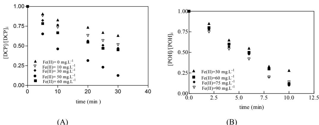
Figure 7.29: DCP and POH degradation as function of time for different Fe (II) initial concentration. (A)  $[H_2O_2]_i = 10 \text{ mg.L}^{-1}$  and experimental time 40 min. (B)  $[H_2O_2]_i = 50 \text{ mg.L}^{-1}$  and experimental time 15min and free pH evolution.
