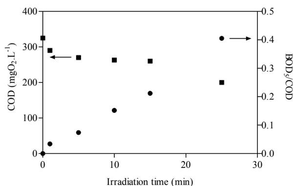
Figure 10.12: Evolution of BOD<sub>5</sub>/COD and COD Vs irradiation time for textile industrial water
