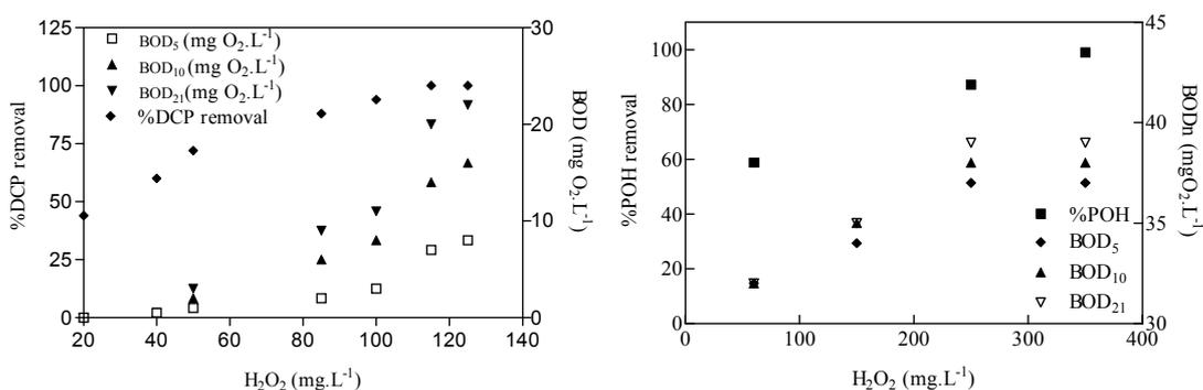
Figure 7.16:  $\text{BOD}_n$ , DCP removal and POH removal removals percentage evolution as function of initial  $\text{H}_2\text{O}_2$  in modified Fenton reaction.  $[\text{Fe}(\text{III})]_i = 10 \text{ mg}\cdot\text{L}^{-1}$ , 60 min reaction time (30 min for POH) and free pH evolution
