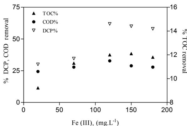
Figure 8.12 DCP, COD and TOC removal as function of initial Fe(III) in UVA/Fe(III) process in single lamp reactor reaction time 90 min.
