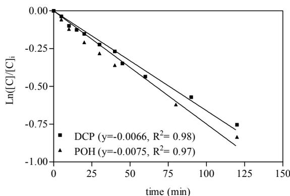
Figure 7.2: first order kinetic constant for DCP and POH degradation by direct UV photolysis
