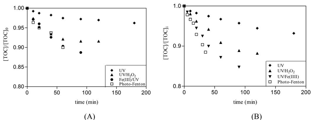
Figure 8.52: Normalized TOC concentrations as function of time for the different AOP's processes, A) single lamp, B) multi lamps reactor.  $[H_2O_2]_i = 50 \text{ mg.L}^{-1}$ ,  $[Fe(III)]_i = 70 \text{ mg.L}^{-1}$ ,  $[Fe(II)]_i = 10 \text{ mg.L}^{-1}$  and free pH evolution.
