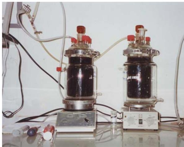
Figure 5.6 biological stirred tank reactors
