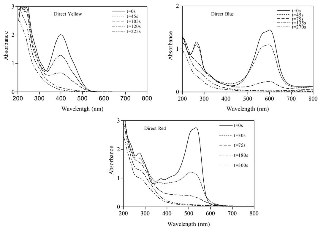
Figure 10.5 : UV photolysis of Optical dyes ( $100 \text{ mg.L}^{-1}$ ).
