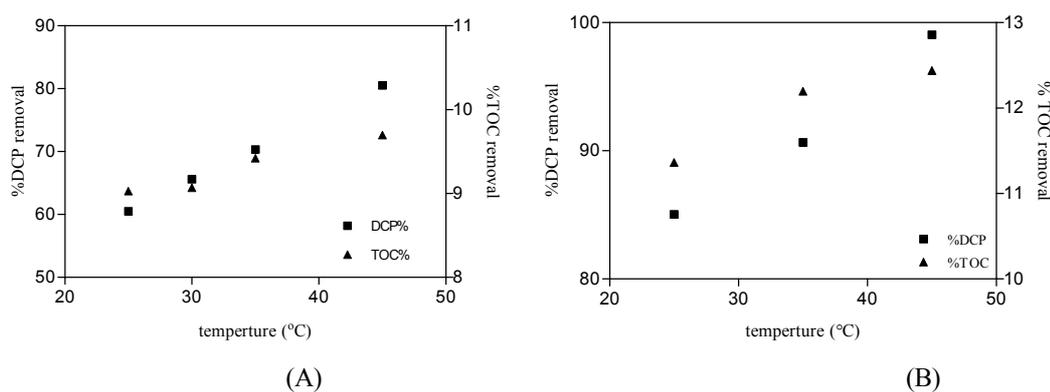
Figure 8.27: DCP% removal and TOC elimination for different initial temperature. A) single lamp reactor,  $[H_2O_2]_i = 30 \text{ mg.L}^{-1}$ ,  $[Fe(II)]_i = 10 \text{ mg.L}^{-1}$ , free pH evolution and reaction time 50 min B) multi lamps reactor,  $[H_2O_2]_i = 30 \text{ mg.L}^{-1}$ ,  $[Fe(II)]_i = 10 \text{ mg.L}^{-1}$ , free pH evolution and reaction time 35 min
