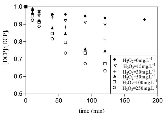
Figure 8.1 Evolution of DCP and TOC as function of UVA-light irradiation time in the single lamp reactor with different initial  $H_2O_2$  concentrations.
