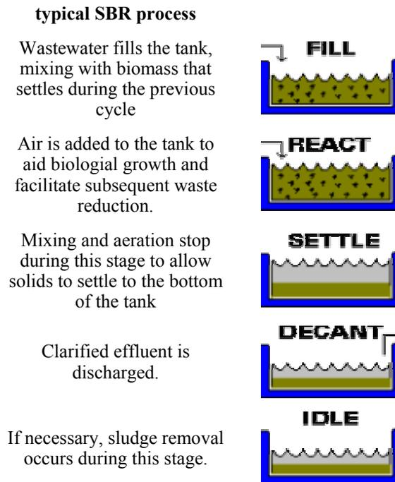
Figure 3.3: SBR process operation steps:
