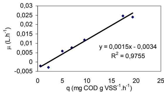
Figure 7.60: Evaluation of  $Y_{X/S}$  and  $k_d$  in the aerobic biological degradation for photo-Fenton pre-Treated solution. Initial conditions 100 mg.L<sup>-1</sup> POH, 50 mg.L<sup>-1</sup> H<sub>2</sub>O<sub>2</sub>, 75 mg.L<sup>-1</sup> Fe (II).
