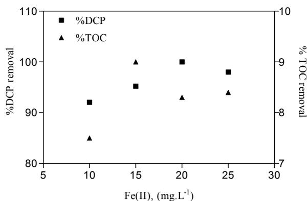
Figure 8.25: DCP and TOC degradation as function of iron initial concentration in single lamp photo-reactor.  $[H_2O_2]_i = 50 \text{ mg.L}^{-1}$  and 50 min irradiation.
