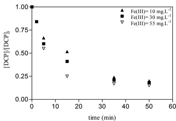
Figure 8.23: Evolution of normalized DCP concentration as function of time at different initial Fe(II) concentration in single lamp reactor.  $[H_2O_2]_i = 30 \text{ mg.L}^{-1}$
