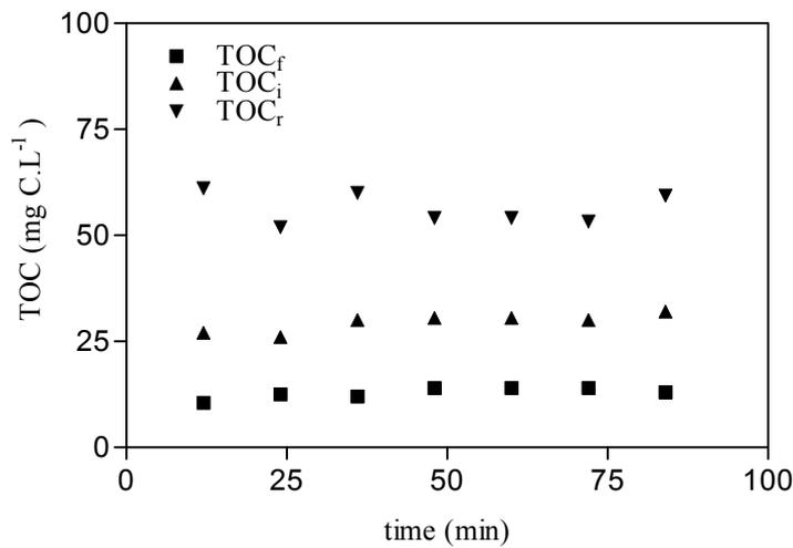
Figure 7.54: Initial, final and TOC removed for the acclimated reactor operating at 100% of photo-Fenton pre-treated solution and HRT = 12 hours.
