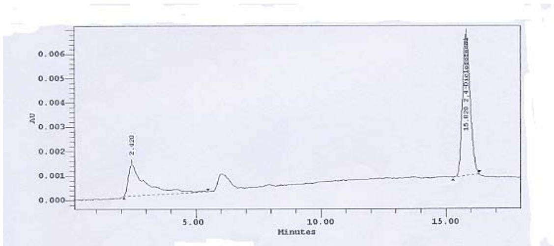
Figure 7.67: Chromatogram corresponding to sample at 30 min of direct UV/Fe(III)
