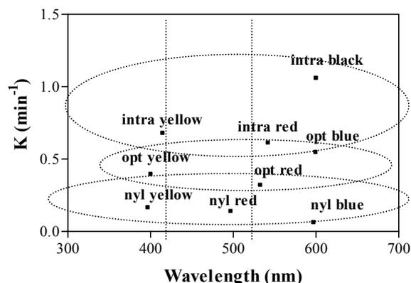
Figure 10.10 : Apparent kinetic constants vs.  $\lambda_{max}$  in the visible range.
