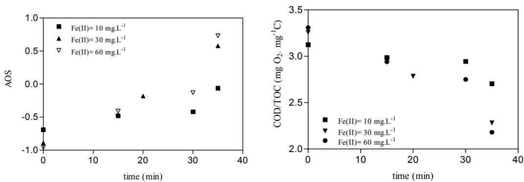
Figure 8.46: AOS and COD/TOC as function of time at different initial Fe(II) in multi lamps photo-reactor.  $[H_2O_2]_i = 15 \text{ mg.L}^{-1}$ , 50 min irradiation time and free pH evolution.
