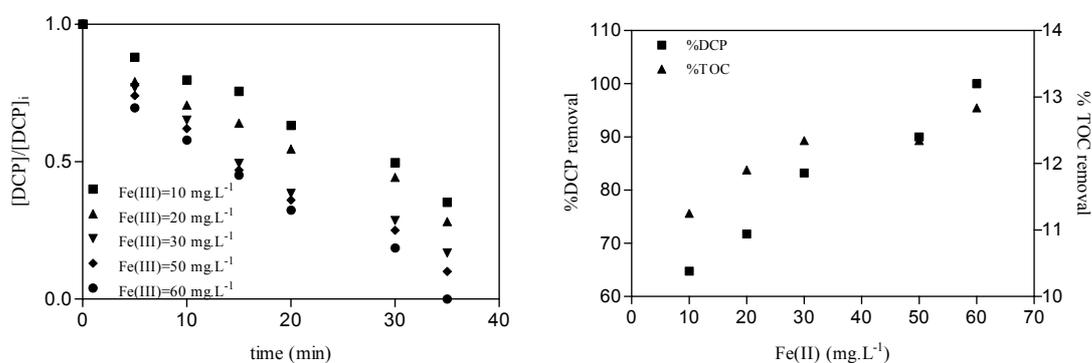
Figure 8.26: DCP degradation as function of iron catalyst in photo-Fenton process in multi lamps reactor.  $[\text{H}_2\text{O}_2]_i = 15 \text{ mg.L}^{-1}$  and 35 min irradiation.
