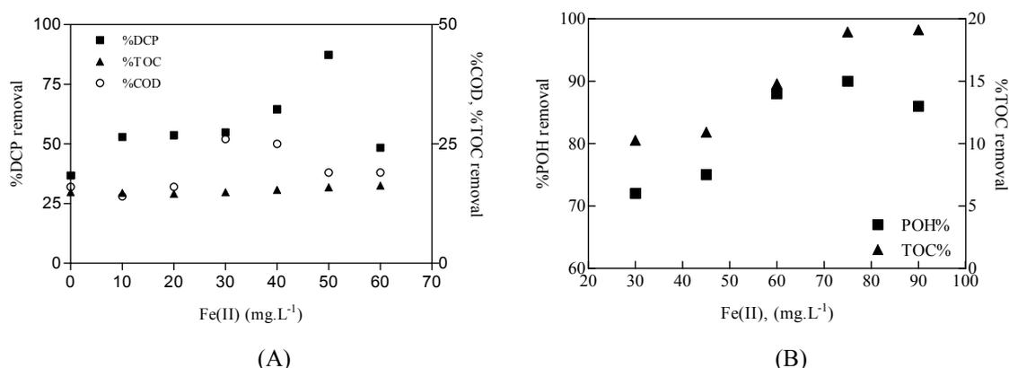
Figure 7.30: DCP, POH and TOC removal percentages as function of initial Fe(II). (A)  $[H_2O_2]_i = 10 \text{ mg.L}^{-1}$  and reaction time 40 min. (B)  $[H_2O_2]_i = 50 \text{ mg.L}^{-1}$  and reaction time 15min and free pH evolution.
