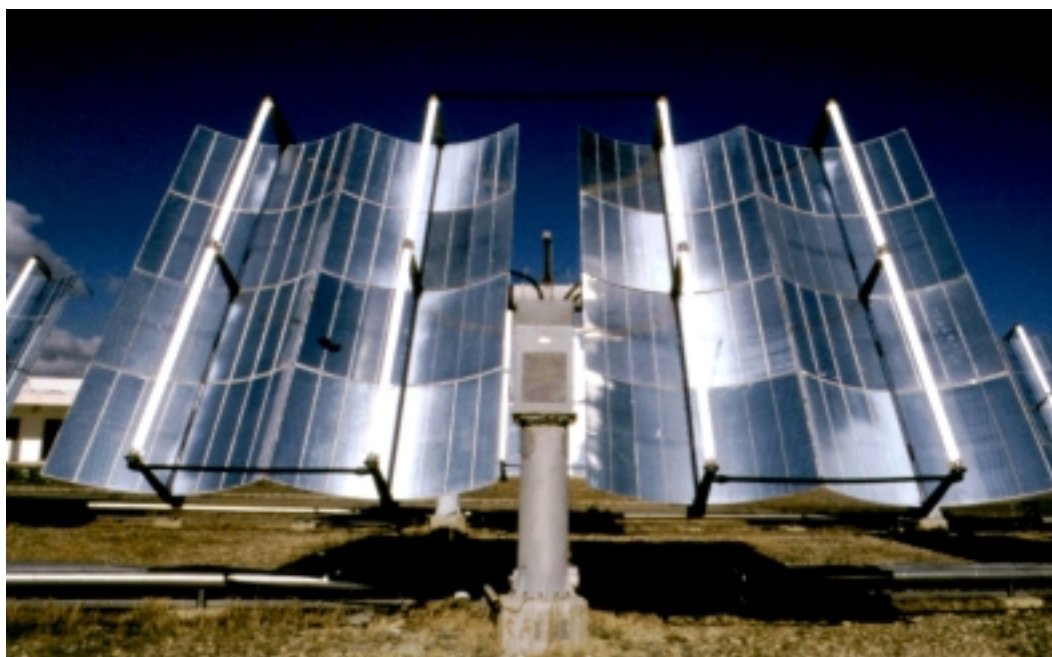
Figure 4.9. Two-axis tracking Parabolic Trough Collector (PTC)
