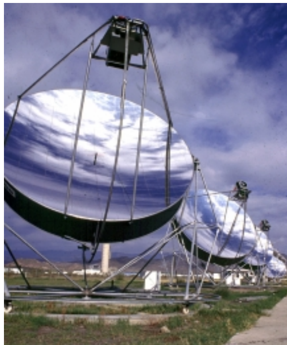
Figure 4.8. High concentrating solar collector. Parabolic dish solar collector (PSA, Spain)
