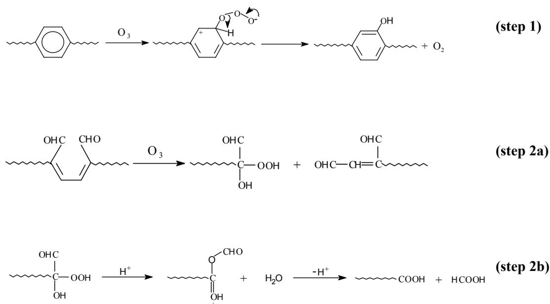
**Figure 4-31 - Direct and anomalous mechanisms of ozonation**
