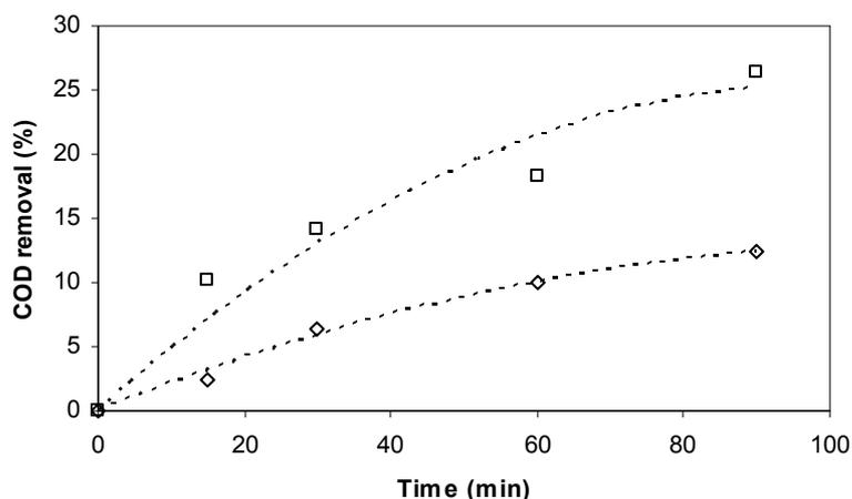
**Figure 4-13 – COD removal vs. time for the ozonation of 50 mg L<sup>-1</sup> (in TOC) solution of (□)18 and (◇)16-BAC. Ozone flow rate 5.44 g h<sup>-1</sup>.**
