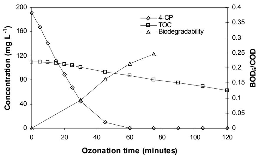
Figure 4-6 - Ozonation of a 200 mg L<sup>-1</sup> 4-CP solution with a 7.57 g h<sup>-1</sup> of ozone flow rate.
