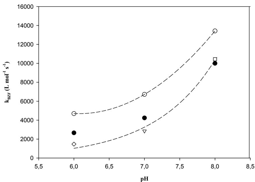
**Figure 4-35 - Kinetic constant values for the BZF ozonation versus pH obtained by means of absolute method (●) and calculated using the literature data for maleic acid reported in table 3 (○: Caprio et al., 1987; ◇:Hoignè and Bader, 1983; ▽: Benkelkacem et al., 2003; □: Pryor et al., 2004).**
