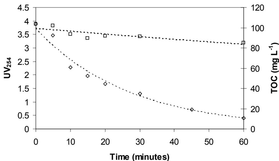
**Figure 4-25 - UV<sub>254</sub> absorbance (◇) and TOC (□) vs. time for the ozonation of SMX. 20 °C and pH no adjusted**
