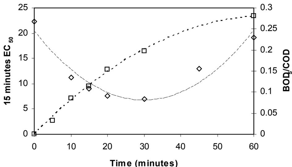
**Figure 4-22 - Biodegradability and toxicity evolution for the SMX ozonation. □ = Ratio BOD<sub>5</sub>/COD; ◇ = 15 minutes EC<sub>50</sub>. 20 °C and pH no adjusted.**
