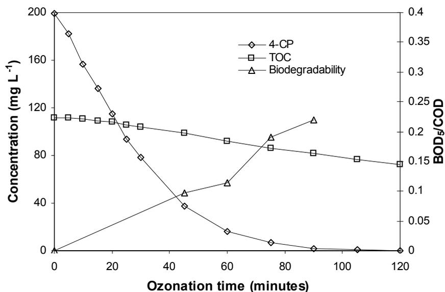
Figure 4-5 - Ozonation of a 200 mg L<sup>-1</sup> 4-CP solution with a 5.44 g h<sup>-1</sup> of ozone flow rate.
