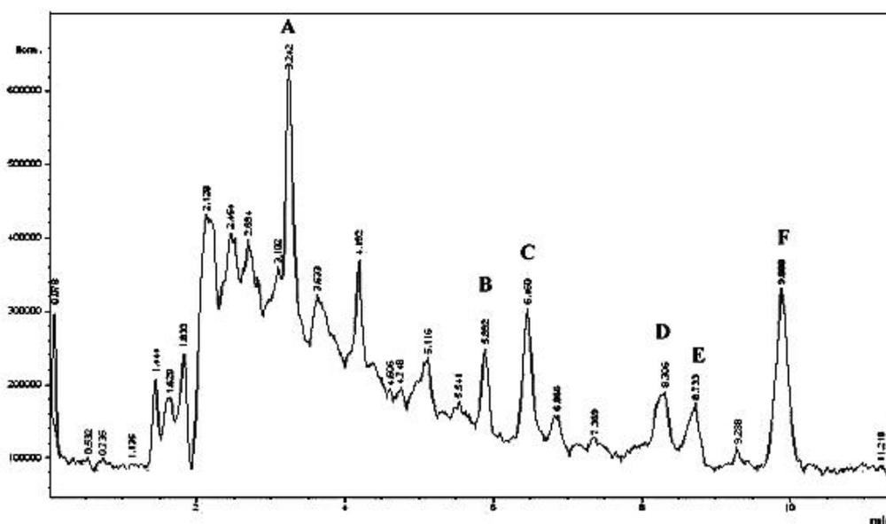
**Figure 4-30 - Chromatogram recorded during LC-MS analysis of the sample collected at 5 minutes of ozonation.**
