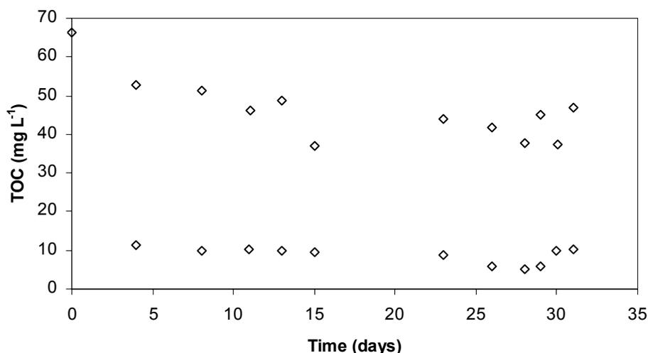
**Figure 4-9 – Initial (15 minutes) and final TOC measurement during biological treatment (SBBR) of pre-treated 4-CP solutions.**
