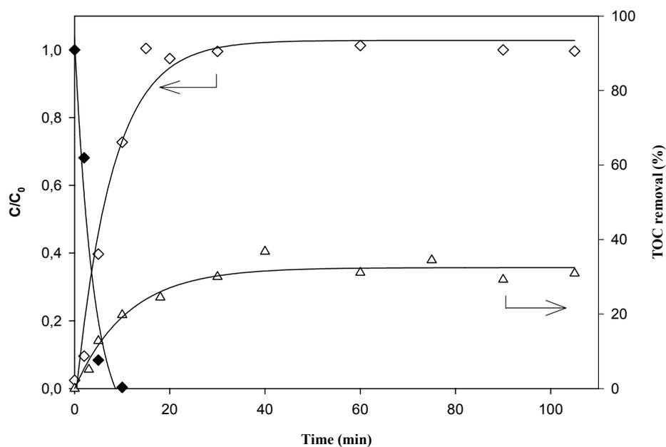
**Figure 4-29** Ozonation of bezafibrate,  $T = 25 \text{ }^\circ\text{C}$   $\text{pH} = 6.0$ ;  $\blacklozenge$  = BZF concentration;  $\diamond$  = Chloride release;  $\triangle$  = TOC removal.
