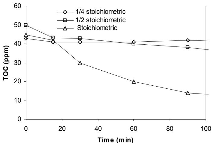
**Figure 4-16 - Mineralization of 18-BAC solutions by photo-Fenton process at different  $\text{H}_2\text{O}_2$  concentration (initial pH = 6,  $[\text{Fe}] = 20 \text{ mg L}^{-1}$ ,  $T = 25 \text{ }^\circ\text{C}$ ).**
