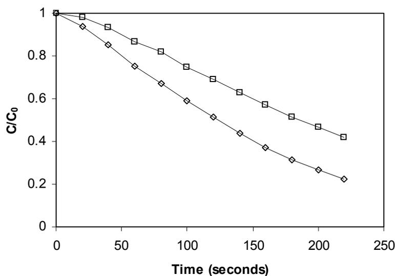
**Figure 4-26 - Ozonation of SMX 0.5 mmol L<sup>-1</sup> + FA 0.5 mmol L<sup>-1</sup>. 20 °C, I = 0.1 M, pH = 5. □ = FA; ◇ = SMX.**
