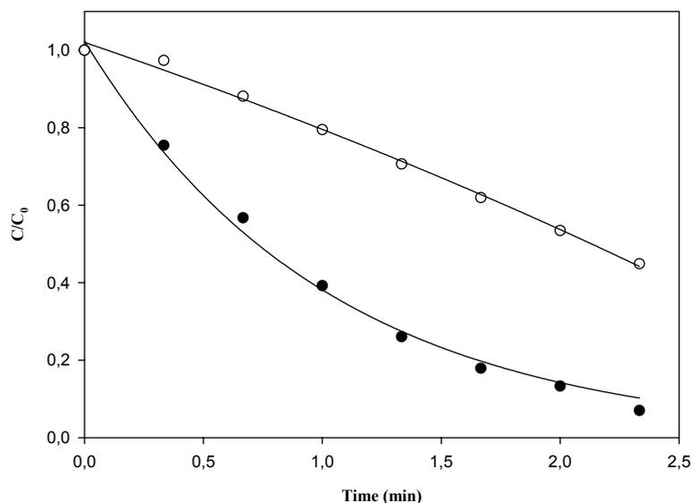
**Figure 4-34 - Normalized concentration of BZF (○) and MAL (●) versus time. Buffered at pH = 6.0. T = 25°C, Ionic strength = 0.1 mol L<sup>-1</sup>.**
