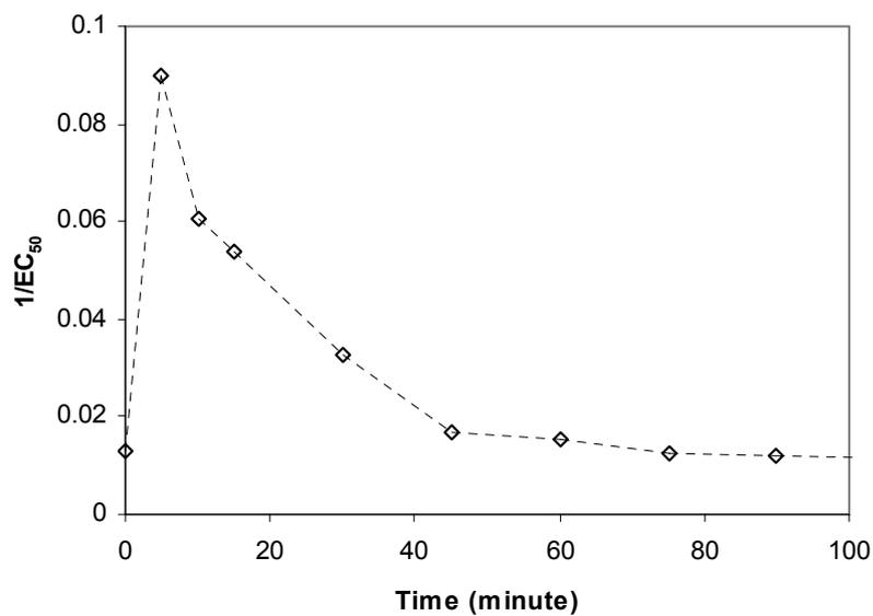
Figure 4-33 -  $1/EC_{50,15 \text{ min}}$  from Microtox<sup>®</sup> test vs. time for the BZF ozonation.
