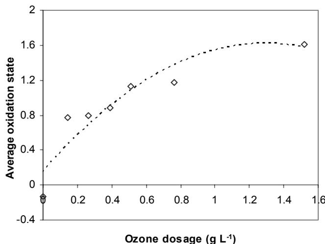
**Figure 4-24 – Average oxidation state measurements during the ozonation of a 200 mg L<sup>-1</sup> SMX solution. 20 °C and pH no adjusted.**
