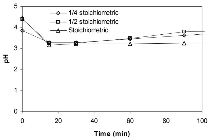
**Figure 4-17 - PH evolution during mineralization of 16-BAC by photo-Fenton with UV lamp**
