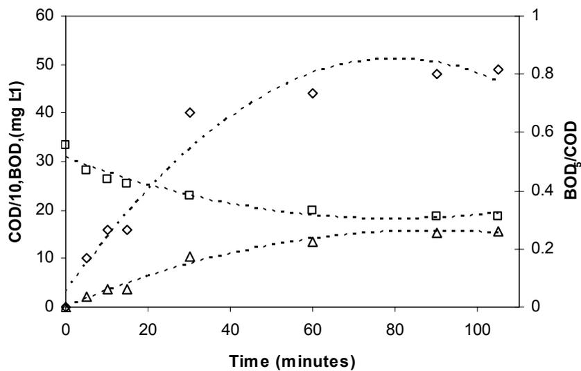
Figure 4-32 - Biodegradability increment during the ozonation of BZF.  $\diamond$ : BOD<sub>5</sub>;  $\square$ : COD;  $\triangle$ : BOD<sub>5</sub>/COD.
