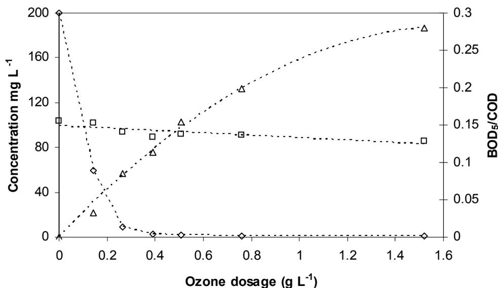
**Figure 4-20 - Ozonation of sulfamethoxazole.  $\diamond$  = SMX concentration;  $\square$  = TOC concentration;  $\Delta$  = ratio BOD<sub>5</sub>/COD. 20 °C and pH no adjusted.**
