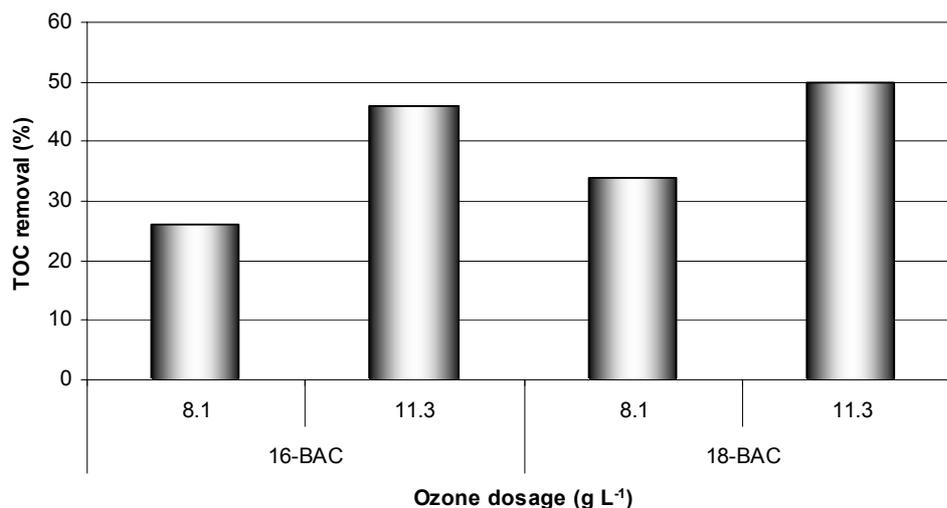
**Figure 4-12 - TOC removal of 16 and 18-BAC after 90 minutes of ozonation.**
