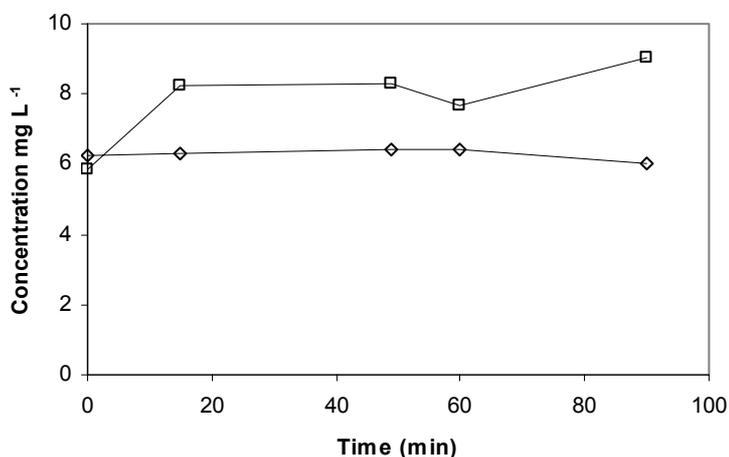
**Figure 4-14 – Ozonation of  $10 \text{ mg L}^{-1}$  (in TOC) 16-BAC solution. pH =  $\diamond$ ; 16-BAC concentration =  $\square$ . Ozone flow rate of  $5.44 \text{ g h}^{-1}$ .**
