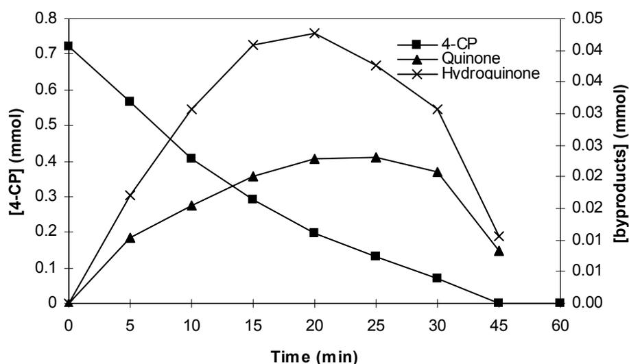
**Figure 4-7 - Quinone and hydroquinone formation during ozonation of a 100 mg L<sup>-1</sup> 4-CP solution with a 7.57 g h<sup>-1</sup> of ozone flow rate.**
