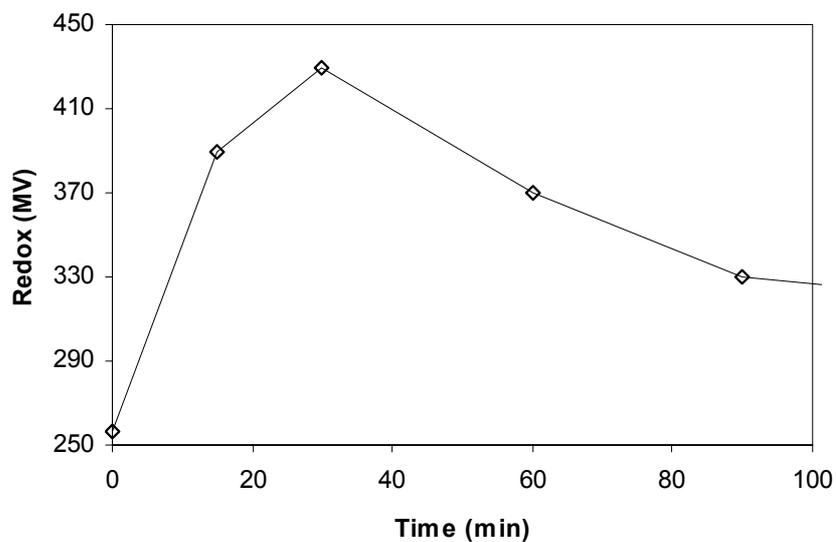
**Figure 4-18 - ORP evolution during mineralization of 16-BAC by photo-Fenton (UV lamp) with 1/2 stoichiometric  $H_2O_2$  concentration.**
