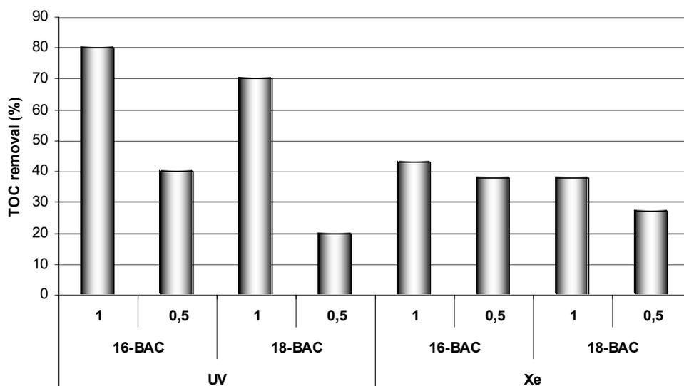
**Figure 4-19 - TOC removal after 90 minutes of photo-Fenton treatment with different ratio  $H_2O_2$ /surfactant (mol/mol).**
