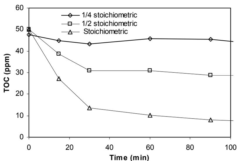
**Figure 4-15 - Mineralization of 16-BAC solutions by photo-Fenton process at different  $\text{H}_2\text{O}_2$  concentration (initial pH = 6,  $[\text{Fe}] = 20 \text{ mg L}^{-1}$ ,  $T = 25 \text{ }^\circ\text{C}$ ).**
