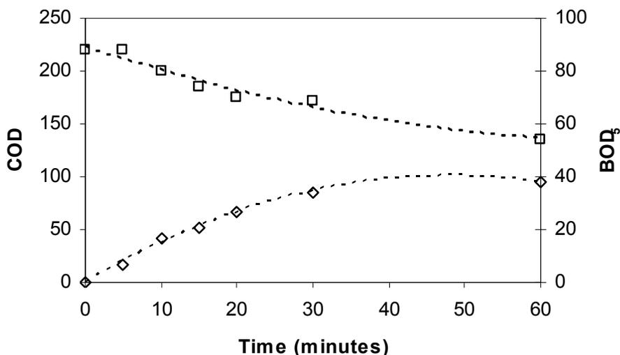
**Figure 4-21 - Ozonation of sulfamethoxazole.  $\diamond$  = BOD<sub>5</sub> (mg O<sub>2</sub> L<sup>-1</sup>);  $\square$  = COD (mg O<sub>2</sub> L<sup>-1</sup>). 20 °C and pH no adjusted.**
