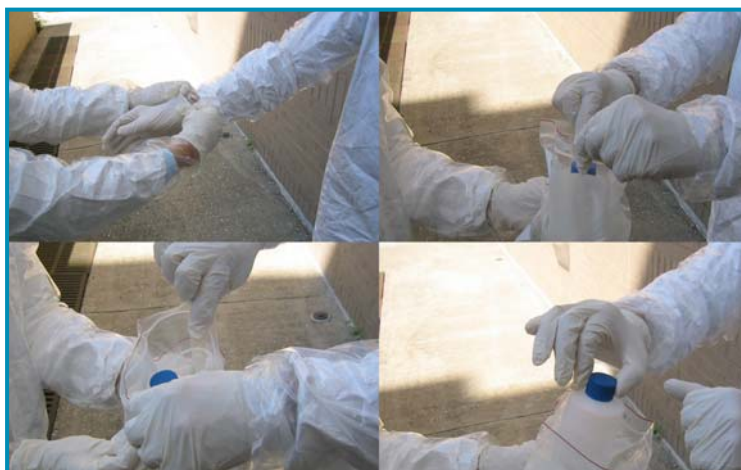
Figure 1.4.5. 'Clean hands/dirty hands' technique. 'Dirty hands' sampler is not in direct contact with the sample. 'Clean hands' sampler is only in direct contact with the sample or cleaned items. Pictures: T. Frick. Técnica 'manos limpias / manos sucias'.
