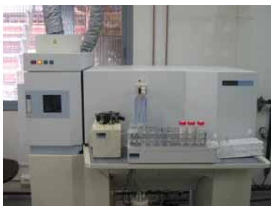
Figure 29: Perkin Elmer Elan Optima 3200 RLs (left). Flame obtained by ICP_OES (right).
