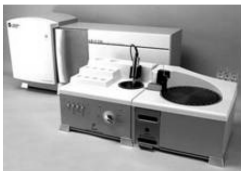
Figure 33: Beckman Coulter (model LS 13, 320) particle size laser analyser.
