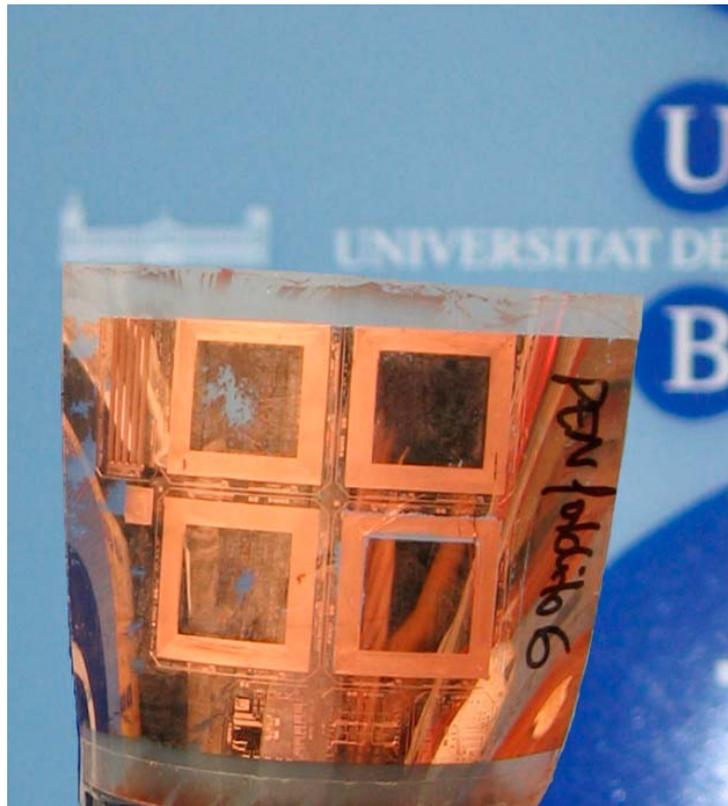
Figure 4.15: Image of copper coils obtained over PEN/seed layer substrate
