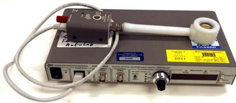
Figure 3.7: Photograph of EQCM and the support to work in liquids containing the quartz crystal resonators metallised with gold electrodes by vapour deposition
