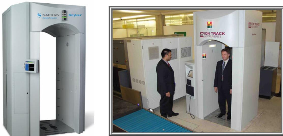
Figure 1.4. IMS portals for drug and narcotic detection provided by Morpho Detection.
