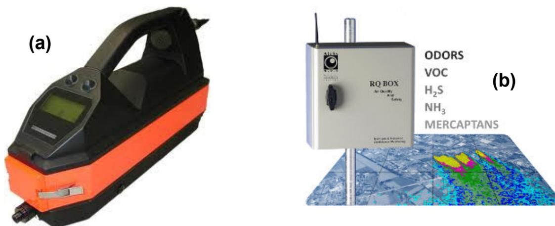
**Figure 1.15.** Commercial instruments which include different sensing technologies. (a) (GDA2) by Airsense Analytics includes an ion mobility spectrometer (IMS), a PID, an electrochemical cell (EC) and 2 MOXs. (b) (RQbox) by Alpha MOS is a field based e-nose for odour and pollutant gases monitoring. It includes an EC, a PID and different MOXs.
