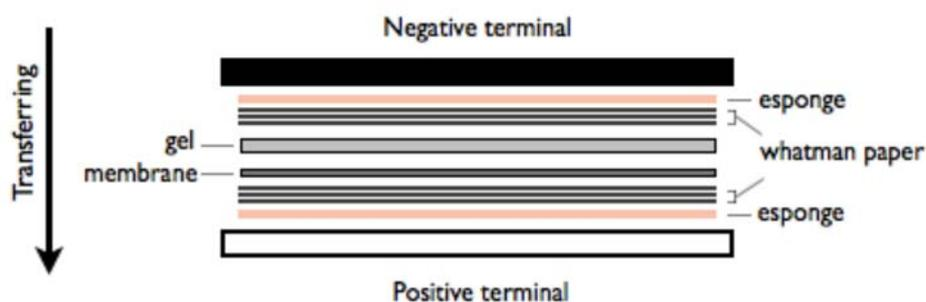
Figure 1 Transferring assembling for western blotting.
