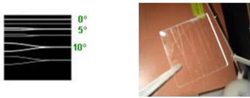
FIG. 8: The left picture is the acetate mask and at the right it can be seen the pattern of SU8-10 above the borosilicate crystal.
