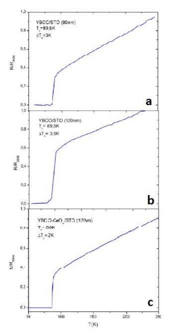
**FIG. 7:** R(T) measurements of a) YBCO 80nm, b)YBCO 120nm, c) YBCO-CeO<sub>2</sub> 120nm
