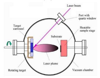
FIG. 1: Standard PLD chamber.
