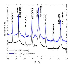
**FIG. 2:** Diffractograms of  $2\theta$ - $\omega$  scans of samples grown on STO.
