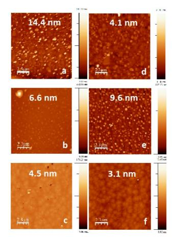
FIG. 6: Morphology and RMS value (top) of a) YBCO 120nm on STO, b) YBCO 80nm on STO, c) YBCO-CeO<sub>2</sub> 120nm on STO, d) YBCO 120nm on LAO, e) YBCO 80nm on LAO, f) YBCO-CeO<sub>2</sub> 120nm on LAO.
