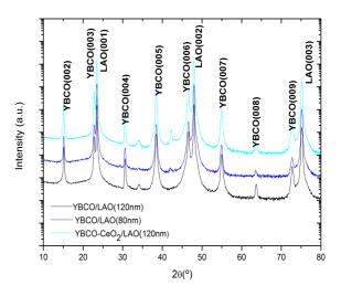
**FIG. 3:** Diffractograms of  $2\theta$ - $\omega$  scans of samples grown on LAO.
