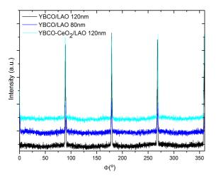
**FIG. 5:** XRD  $\Phi$ -scans around asymetrical YBCO(308) reflection for samples grown on LAO.
