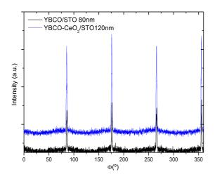
**FIG. 4:** XRD  $\Phi$ -scan around asymetrical YBCO(308) reflection for samples grown on STO.
