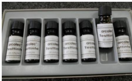
Figure 4. Testing inks for different measures of surface tension.
