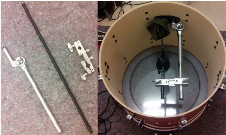
Figure 6.7. Left to right: material used to make the homemade microphone holder, floating microphone system inside the bass drum.
