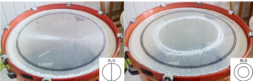
Figure 7.4. Examples of Chladni's patterns seen on the batter drumhead.
