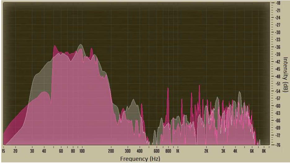
Figure 7.21. Comparison of frequency spectrums: ideal bass drum's sound (white) and C configuration (pink).
