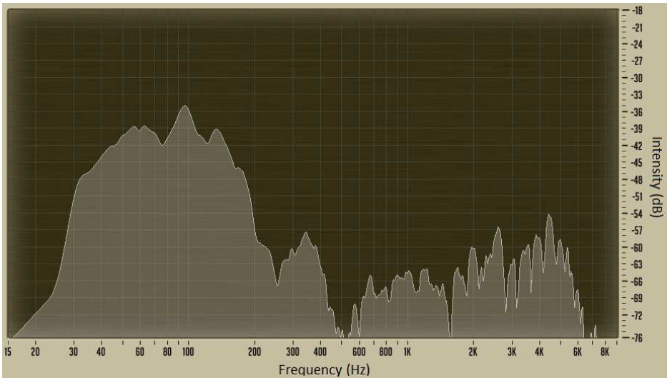
Figure 7.11. Frequency spectrum of the ideal bass drum's sound.
