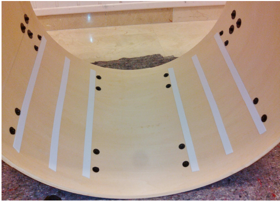
Figure 6.11. EVA foam inside the bass drum.
