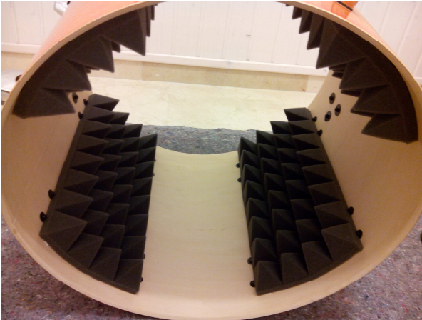
Figure 6.10. Acoustic material improvement for a bass drum.
