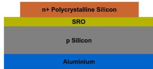
Fig. 1. Schematic view of the fabricated devices (not to scale).
