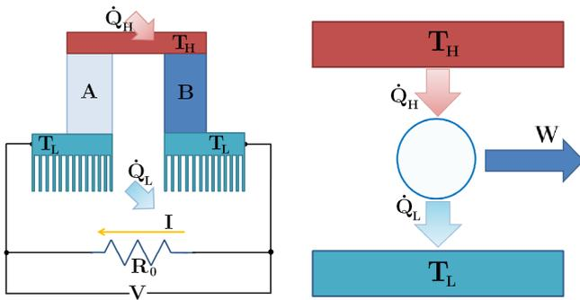
FIG. 1: The behavior of a TE generator corresponds to a heat engine working between a hot source at temperature  $T_H$  and a cold sink at temperature  $T_L$ .
