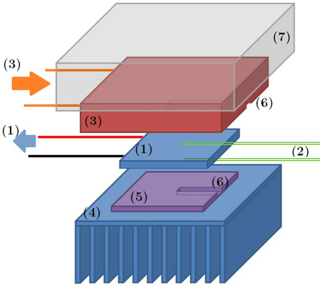
FIG. 2: Simple drawing of the experimental system used to characterize the Peltier module.
