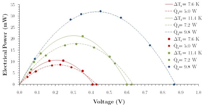
FIG. 7: Power output in front of voltage output. The legend for the markers is the same as in Fig.(6).
