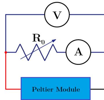
FIG. 4: Circuit used to measure the I-V curves.
