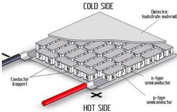
FIG. 3: Schematic diagram of a Peltier cooler. According to The Renewable Energy Website: <http://www.reuk.co.uk/>
