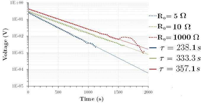
FIG. 5: The y-axis is in logarithmic scale. Three different transient curves were obtained for  $R_0 = 5, 10$  and  $1000 \Omega$ . Dot lines represent the experimental transient curve. Solid lines represent the linear adjustment.
