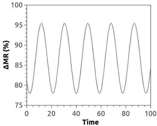
FIG. 7: Variation of the giant magnetoresistance of the contact region with time. Here, 0% represents the maximum conductivity ( $m_z = 1$ ), when the magnetizations of the free and fixed layers are parallel. On the other hand, 100% corresponds to  $m_z = -1$ , and the magnetoresistance is maximal.
