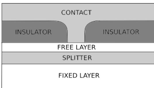
FIG. 3: Simplified version of the spin transfer torque setup. A nanometric hole is performed on an insulating layer (usually  $\text{SiO}_2$ ), thus creating a nanocontact that is used to excite dynamics in the free ferromagnetic layer. The fixed layer is below, with a non magnetic splitter in order to affect the polarization of the moving electrons only.
