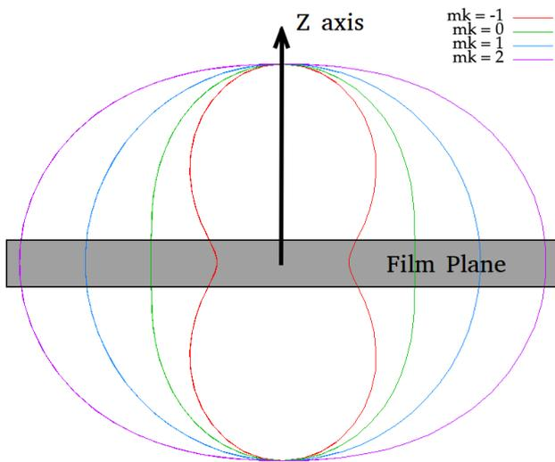
FIG. 4: Anisotropy energy as a function of the polar angle  $\theta$  for different values of the anisotropy parameter  $m_k$ .
