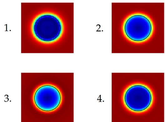
FIG. 6: Color map of the values of  $m_z$  under the nanometric contact. The contact position and shape is shown by the black circumferences. The pulsation, which affects the size and depth of the droplet can be seen.
