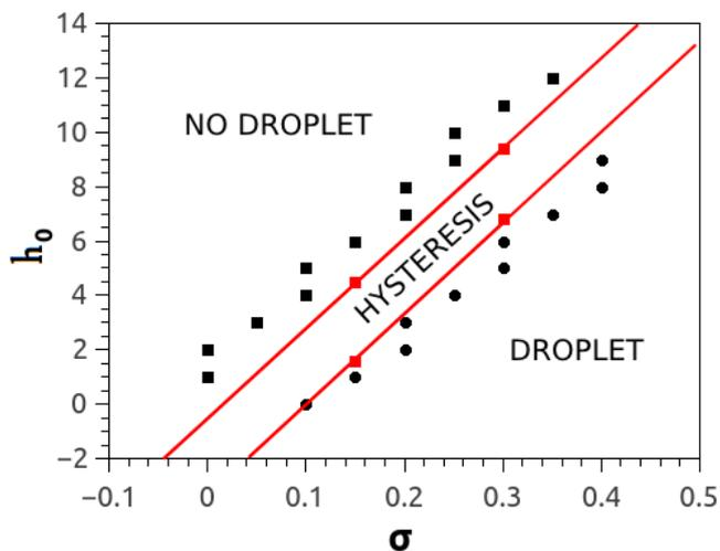
FIG. 5: Regions of stability of the droplets, for different values of the injected current  $\sigma$  and the external magnetic field  $\mathbf{h}_0$ . In the upper region the droplets cannot exist, while in the lower region droplets are always created. There is, however, a thin band between the two regions where the droplets are neither created nor destroyed (hysteretic behavior).
