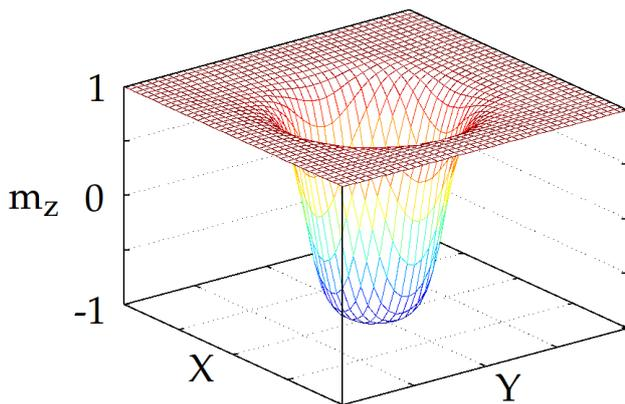
FIG. 1: Example of the result of one simulation. A magnetic droplet soliton has been created and it is stable. Notice that the magnetization is pointing upwards everywhere but below the contact, where it is reversed.
