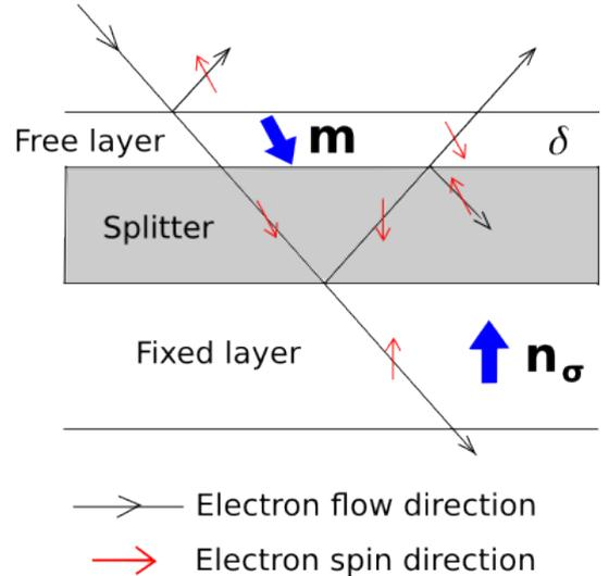
FIG. 2: Working principle of the spin transfer torque. Magnetization is represented by the blue big arrows, and the spin of the electron fluxes is shown as the red thin arrows. In this idealized example, only the electrons with their spin parallel to the magnetization are transmitted through the ferromagnetic layers, while those with antiparallel spin are reflected back.
