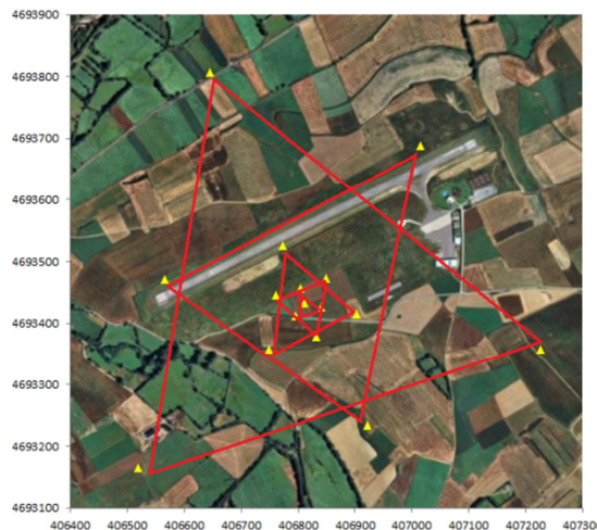
FIG. 3: Final arrays realised in the aerodrome (red). Stations (yellow) expect to be as equidistant from the centre as possible. Absolute coordinates scale [2].
