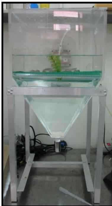
**Figure 1.** Custom made breeding chamber. A grid is located in the bottom in order to avoid predation of the eggs by the parent fishes. Plastic plants and marbles can be placed in the tank in order to stimulate the spawning. The shape of the tank, as a funnel on the bottom, allows simple release of the newly spawned eggs.
