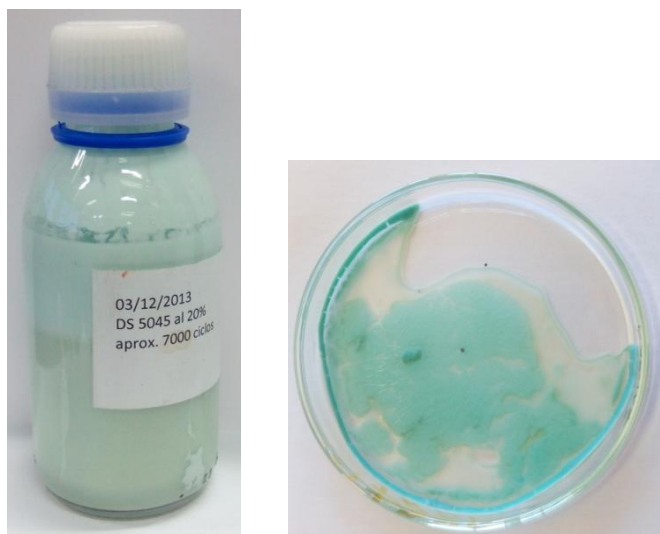
Figure 6. 2. a) Image of the 7000 cycles Micronal ® DS 5045 X sample used for the study untitled “Thermal Cycle Feasibility of Phase Change Slurry”, b) Image of dried Micronal ® DS 5045 X.
