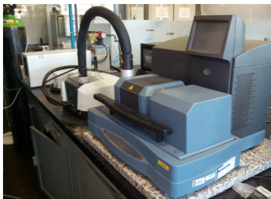
Figure 3.7.- TGA instrument coupled to FT-IR device.
