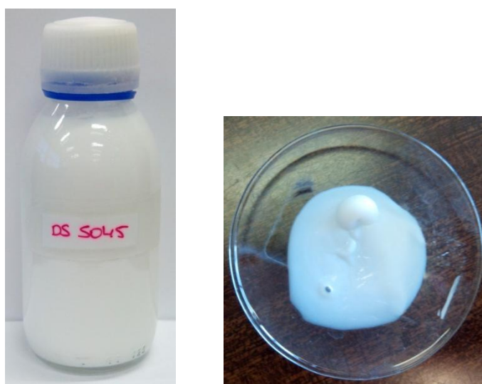
Figure 6. 1. a) Image of Micronal ® DS 5045 X sample used for the study untitled “Thermal Cycle Feasibility of Phase Change Slurry”, b) Image of dried Micronal ® DS 5045 X.
