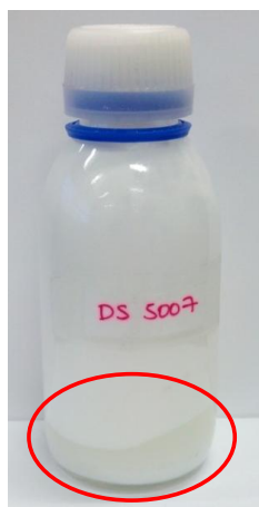
Figure 5.2. Image of Micronal ® DS 5007 X sample used for the study titled “Physicochemical and thermal study of a MPCM of PMMA shell and paraffin wax as a core”.
