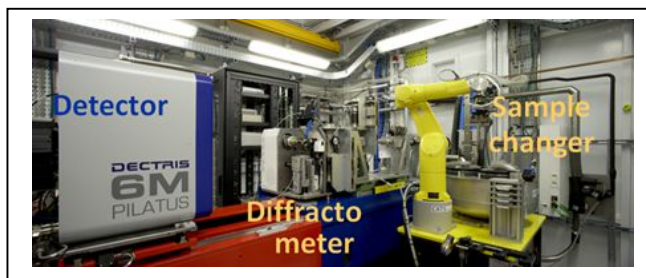
FIG.6. Experimental Hutch of XALOC beamline. The detector is where the diffraction pattern is collected, the diffractometer has all the elements to move and keep the crystal in good conditions under the beam during collection and the sampler changer permit to handle the crystals from control room.
