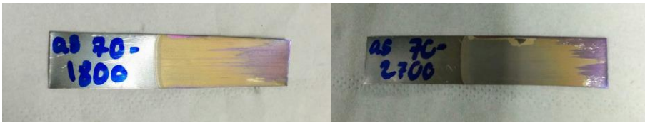
Figure 20. Sample images of non-uniform oxidation at 70V.
