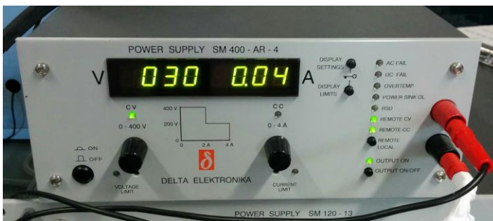
Figure 7. Power supply DELTA ELEKTRONIKA SM 400-AR-4
