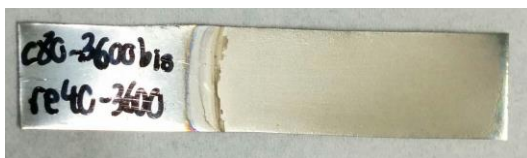
Figure 21. Sample c80-3600re40-3600 two-step anodized.
