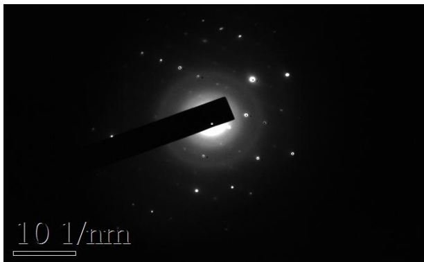
FIG 16: Electron diffraction pattern of the NW of Fig. 15.
