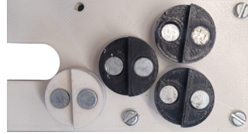
Figure 5.14: 3D parts anchored to the servomotors
