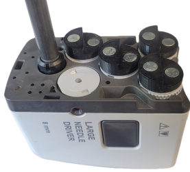
Figure 5.13: 3D parts anchored to the EndoWrist
