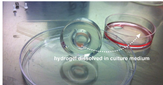
Fig. 53 Image of the casting mold used to fabricate the scaffold, almost without any traces of the PF127 hydrogel with HFF after 24h, incubated at 37 °C 5% CO 2 .
