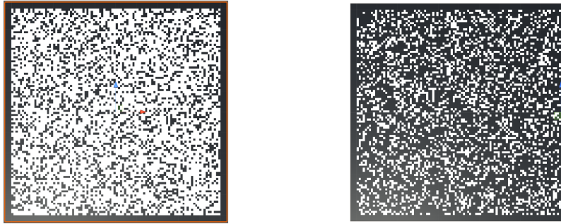
Figure 3.3: Example of what a 100x100 CA would start like if we have a border size of 3, and have our cells start at a random state. Each pixel of the image represents a cell, where black and white pixels are walls and non-wall cells, respectively. On the left, each cell has a 30% chance of being a wall, and on the right, each cell has a 70% chance.
