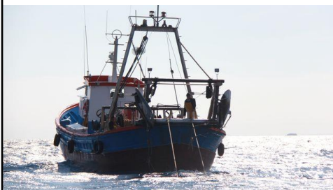
Figure c. Example of Bottom trawler used for harvesting European hake in the Spanish Mediterranean Sea (Eldiariocv.es, 2016).
