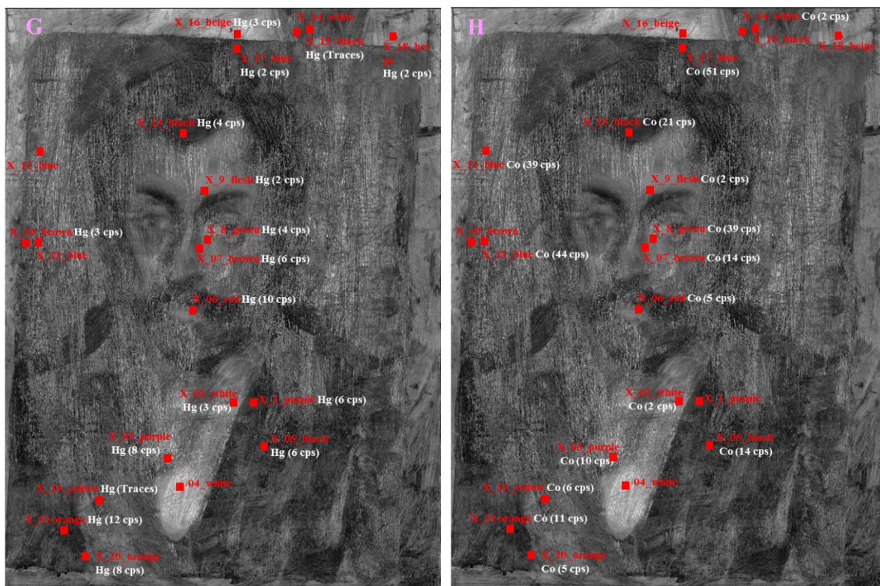
Figure 75. XRF mapping- element distribution and cps obtained: a) Pb, b) Ba, c) Zn, d) Ca, e) Fe, f) Mn, g) Hg, h) Co.
