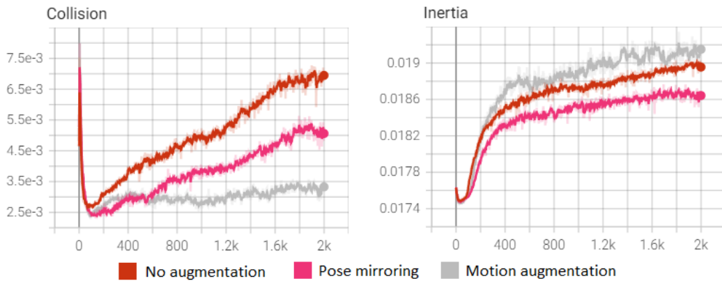
FIGURE 6.7: Data augmentation ablation. Collision (left) and inertia (right) metrics evolution for validation set during training for different augmentation techniques. First: no augmentation. Next: pose mirroring. Finally, a novel motion augmentation technique. The latter is only possible thanks to disentangled encoders. As cloth dynamics are being learnt by the network, collisions slightly increase. Pose mirroring reduces this effect, while motion augmentation mitigates it almost completely. We also see the evolution of cloth dynamics – inertia metric– is not compromised by these changes.
