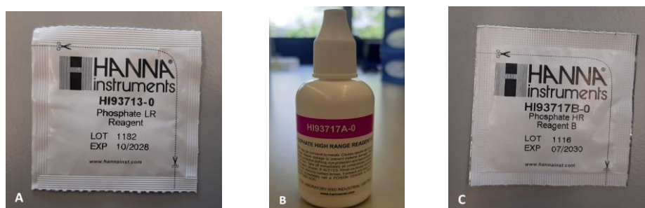
Figure 6. Reagents used for commercial phosphate determination: (A) Hanna Instruments LR Reagent powder packet (HI93713-0); (B) Hanna Instruments HR Reagent A liquid dropper bottle (HI93717A-0); and (C) Hanna Instruments HR Reagent B powder packet (HI93717B-0)
