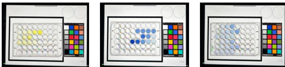
Figure 13. Smartphone-captured images of the colour development profiles for phosphate quantification: laboratory HR approach (left), commercial HR kit (middle), and both LR methods combined within a single image capture (right).
