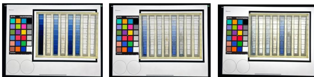
Figure 20. Smartphone digital image captures for real sample quantification: M1 and M2 (left), M3 and M4 (centre), M5 and M6 (right).
