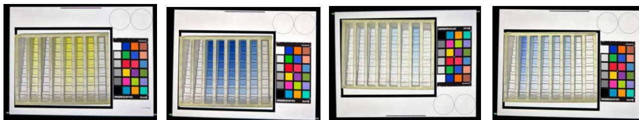
Figure 19. Smartphone-captured images utilizing the simultaneous multi-optical path cell for phosphate quantification across the studied methods. From left to right: laboratory HR (first), commercial HR (second), laboratory LR (third), and commercial LR (fourth).
