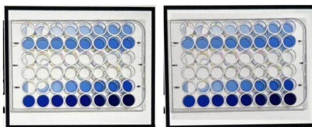
Figure 18. Comparison of the multi-well plate before (left) and after (right) applying the pixel-by-pixel background blank correction.
