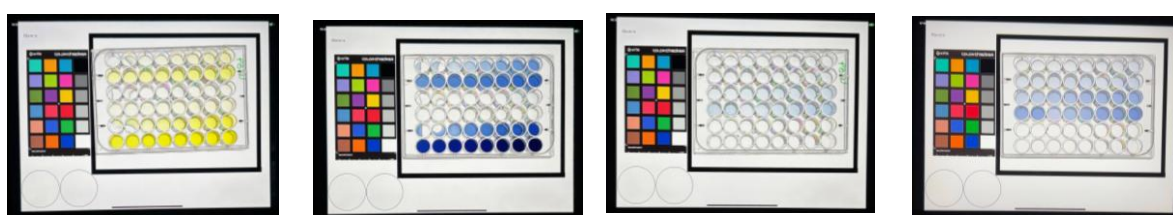
Figure 16. Smartphone-captured images of the volumetric profiling for phosphate quantification. From left to right: laboratory HR (first), commercial HR (second), laboratory LR (third), and commercial LR (fourth).
