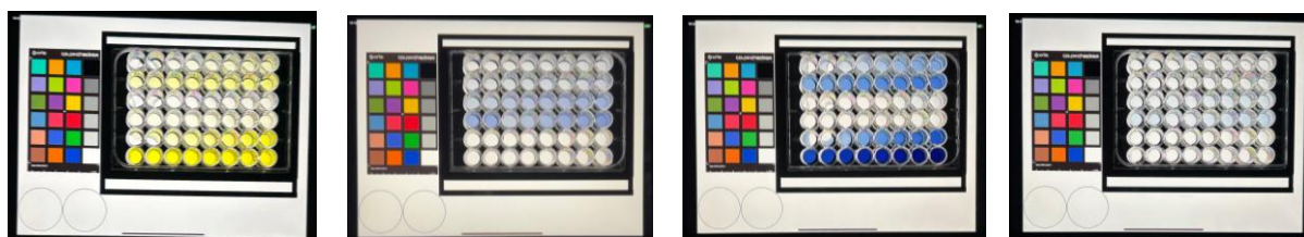
Figure 17. Smartphone-captured images with the illumination mask of the volumetric profiling for phosphate quantification across the studied methods. From left to right: laboratory HR (first), commercial HR (second), laboratory LR (third), and commercial LR (fourth).
