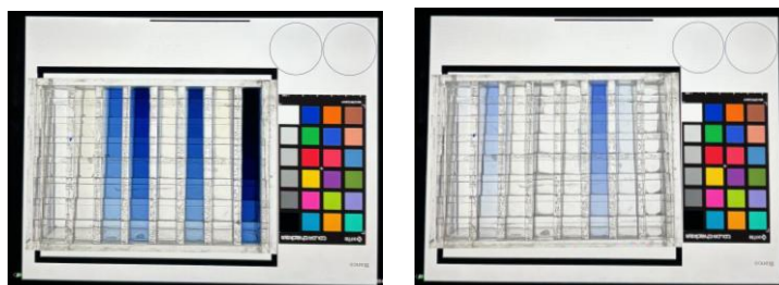
Figure 21. Smartphone digital image captures for real sample quantification utilizing the PMMA-based cell: (left) samples M1 and M2 for HR determination and (right) samples M3 and M4 for LR determination.
