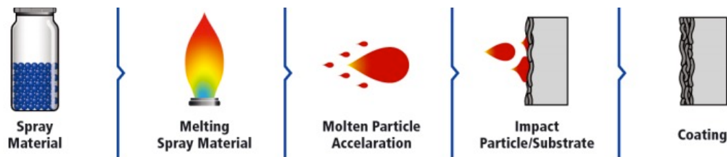
Figure 7. Thermal spray process [44]
