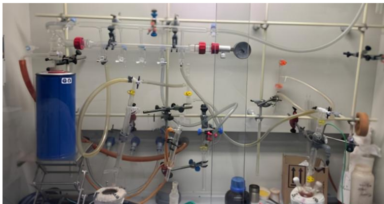
Figure 34. Schlenk line setup used for the colloidal synthesis of CdSe quantum dots under controlled vacuum and nitrogen atmosphere.
