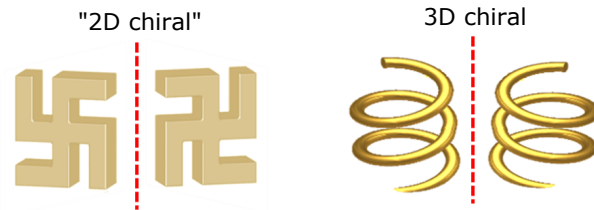
Fig. 1. Pictorial comparison between 2D and 3D chirality. An object (that is not necessarily 2D) is “2D chiral” when it can be brought into congruence with its mirror image when it is lifted from the plane.
