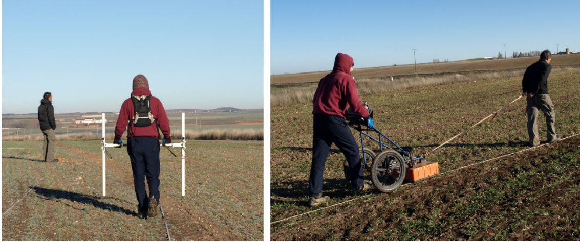
Figure 4.4: Used systems. Bartington gradiometer (left) GSSI GPR equipped with a 270 MHz antenna (right).
