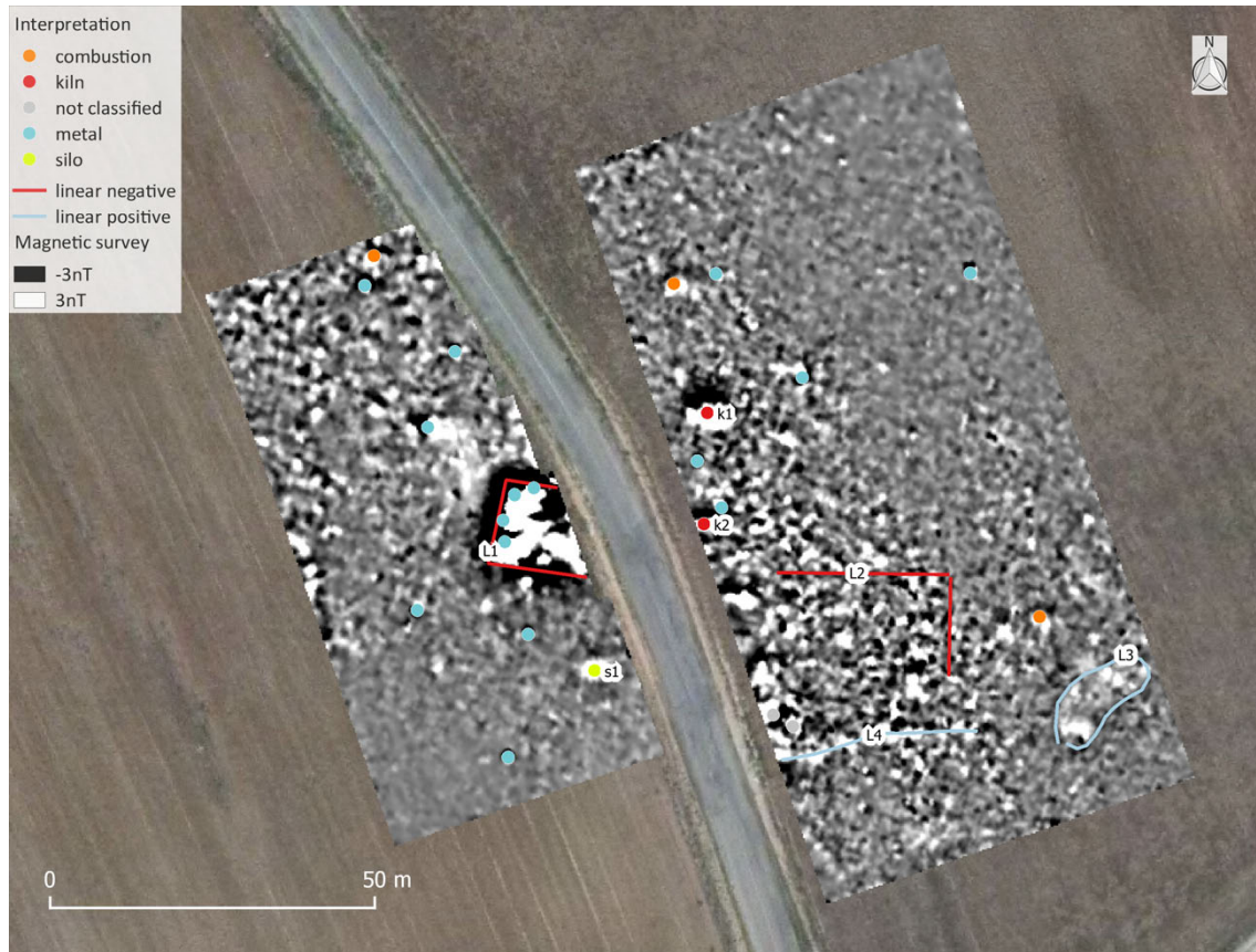
Figure 4.15: Interpretation of the magnetic survey.
