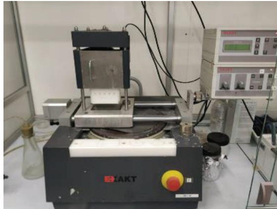
Figure 26: Polishing machine with SiC disc.
