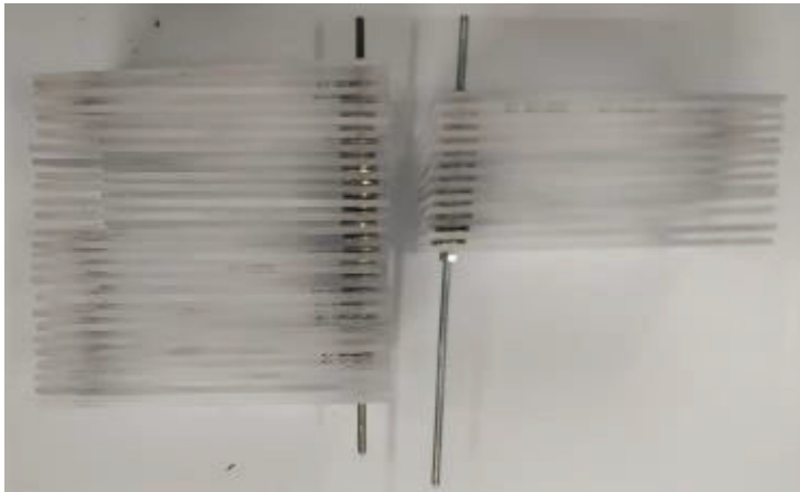
Figure 34: Samples polished to less than 100 \mu\text{m} and placed on the bars to facilitate the staining process.
