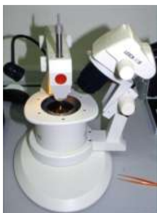
Figure 2. Impact freezing equipments: Leica EM-CPC cooled by liquid nitrogen and Leica Cryoblock, cooled by liquid nitrogen or liquid helium. Both at the CCiT Cryo-EM Laboratory.
