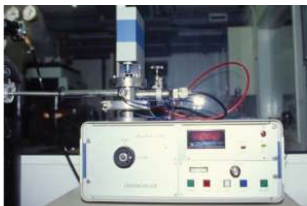
Figure 2. Impact freezing equipments: Leica EM-CPC cooled by liquid nitrogen and Leica Cryoblock, cooled by liquid nitrogen or liquid helium. Both at the CCiT Cryo-EM Laboratory.
