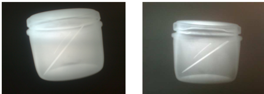
Figure 4: Different radiographic conditions in an experimental example designed by the UTPR-UB for a specific X-ray equipment course. It consists of a jar of food where two thin foreign objects have been detected by means of X-ray technology, showing different image qualities
