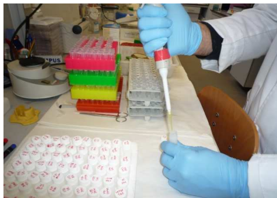
Figure 6: LSC sample preparation for its detection and quantification at a UB Radioactive Facility
