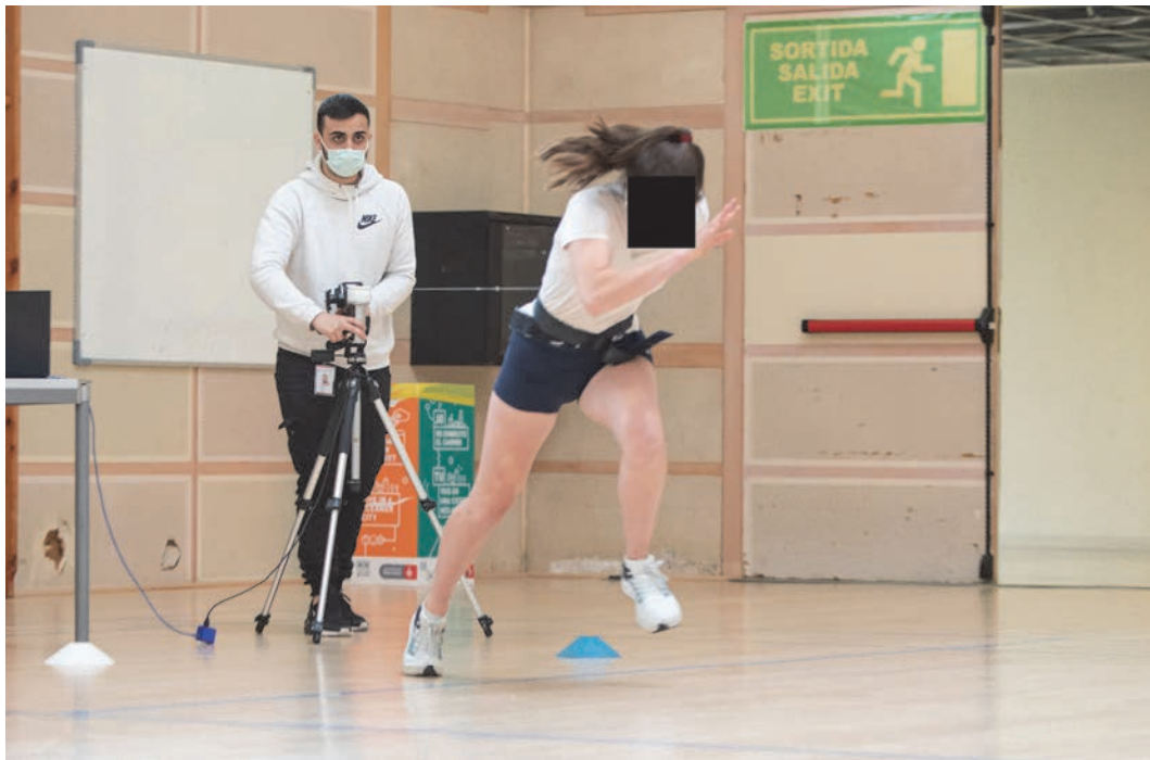
Figure 3.2. Representative illustration showing the sprint performance and mechanical properties assessment using the linear velocity sensor RaceAnalyzer (Chronojump, Barcelona, Spain).
