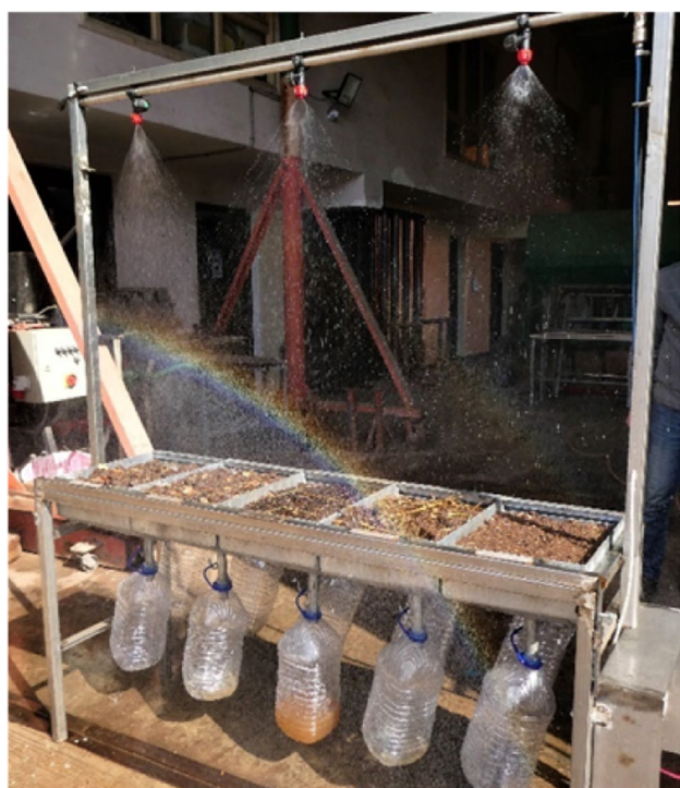
Figure 5 Rainwater simulator developed by INRA is being tested before the Farmer Field Schools (FFS) in Settati, Morocco. Source: Harun Cicek.
