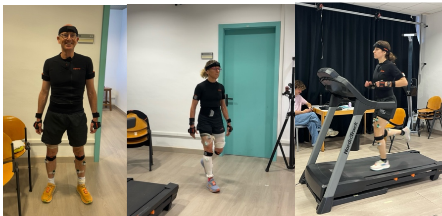
Figure 2. Experimental setup. Left: participant fitted with the Xsens MVN Awinda suit and Delsys Trigno EMG sensors. Centre: IMU calibration procedure before the start of the protocol. Right: participant running on the NordicTrack T11.5 treadmill during data collection.
