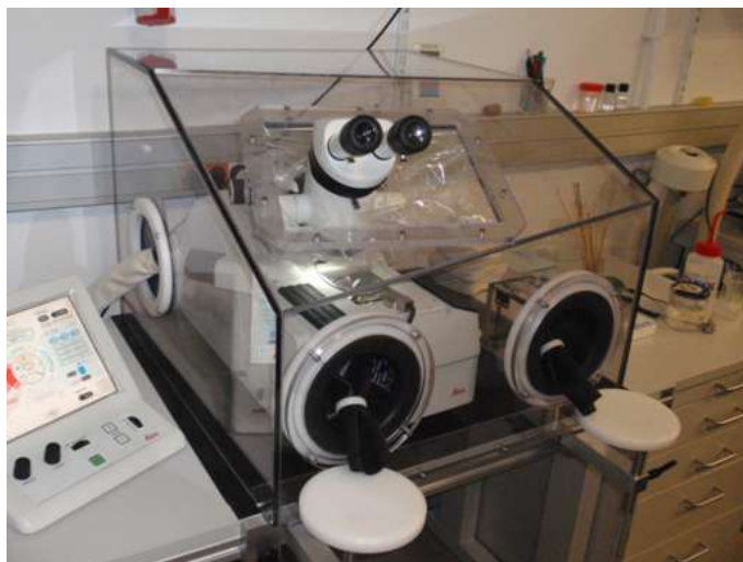
Figure 4. Cryo-ultramicrotome Leica UC6/FC6 with an anti-contamination glove box based on the prototype of Peters Lab. [12], at the CCiTUB Cryo-EM Laboratory.
