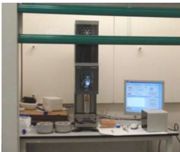
Figure 1. Plunge freezing equipment: Vitrobot Mark III (FEI Company) at the CCiTUB Cryo-EM laboratory.
