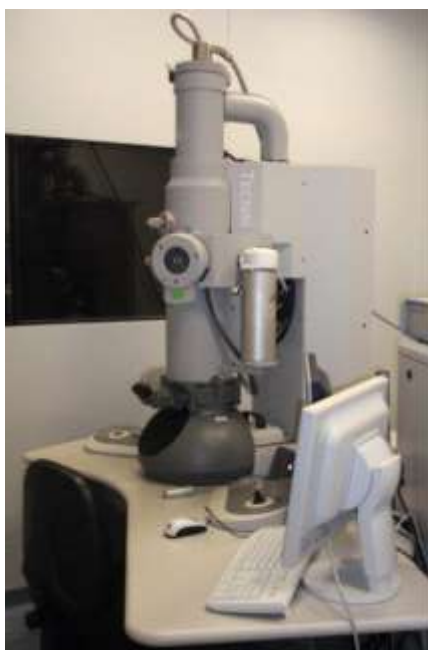
Figure 7. Tecnai Spirit electron microscope, equipped for cryo and tomography at the CCiT Cryo-EM Laboratory.
