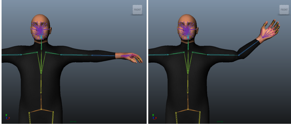
Figure 1.3: The picture on the left shows the mesh without any deformation and the picture on the right shows how the shape of the muscles around the elbow is not preserved when only a slight rotation to start a greeting animation is done
