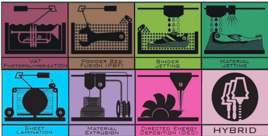
Figure 1: Different types of additive manufacturing printers
