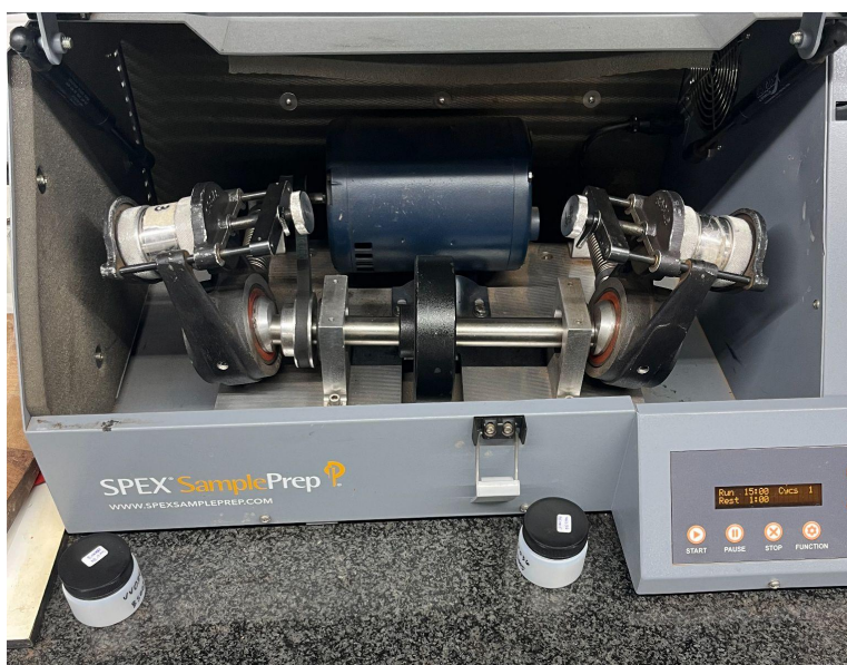
Figure 5. SPEX SamplePrep tungsten ball bearing mill loaded with samples VV0034 and VV0036 (Soler i Gumà, 2025)
