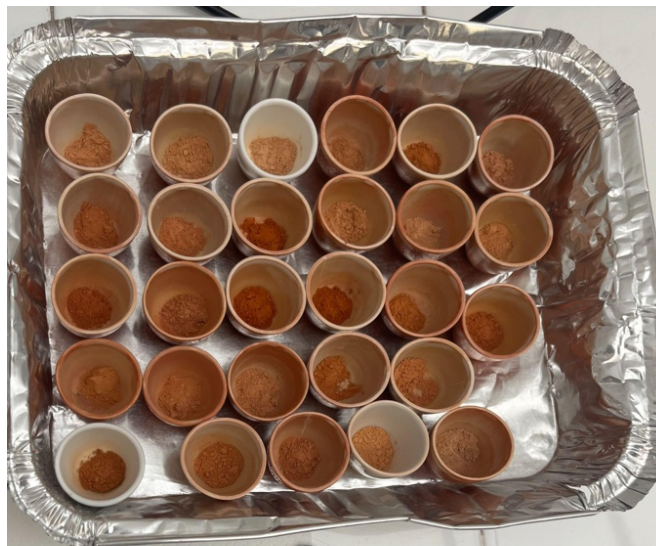
Figure 8. Approximately 0.3 g of each specimen in clay crucibles before loss on ignition test (Soler i Guma, 2026)
