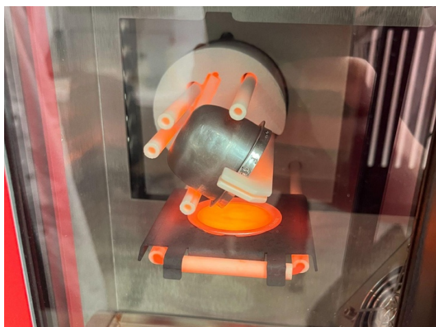
Figure 7. Glass disk during cooling stage after being poured from crucible at 1125°C. These disks will measure the major and minor elements
