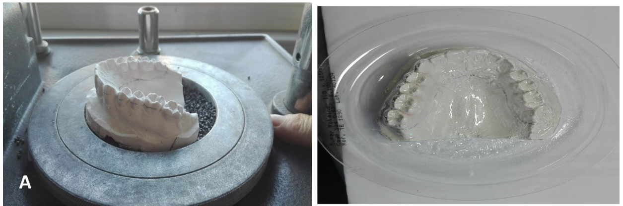
Fig. 12. (A) Cast placed on the vacuum forming machine Biomat. (B) Plastic vacuum adapted over the maxillary cast
