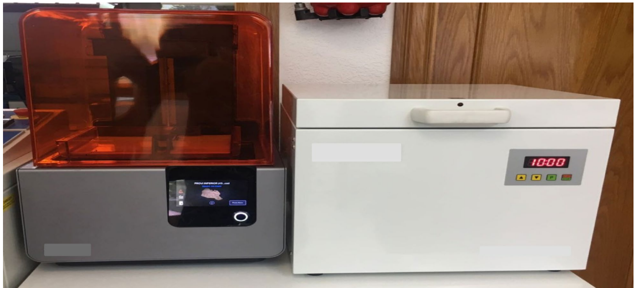
Fig. 23. 3D printing device (Formlab form 2 r ) in the left and light-curing device in the right
