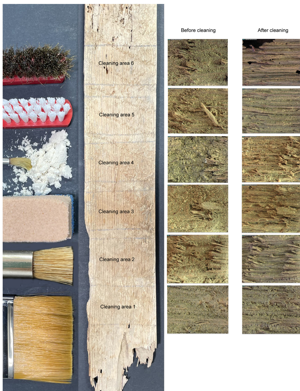
Fig. 5. Comparison of cleaning results with different traditional dry-cleaning tools: long nylon bristle paintbrush and its cleaning results in Area 1; short bristle round paintbrush and its cleaning results in Area 2; Akpad® soft sponge and its cleaning results in Area 3; Milan® 430 powdered eraser and its cleaning results in Area 4; nylon-bristle brush and its cleaning results in Area 5; brass bristle brush and its cleaning results in Area 6 (Dino-Lite® images before and after cleaning at 65\times show wood fibres displayed horizontally for each area).
