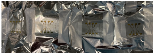
Figure 46: coverslips with electrodes placed on a sheet of aluminum foil.
