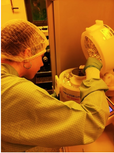
Resin deposition on the wafer inside a spinner
