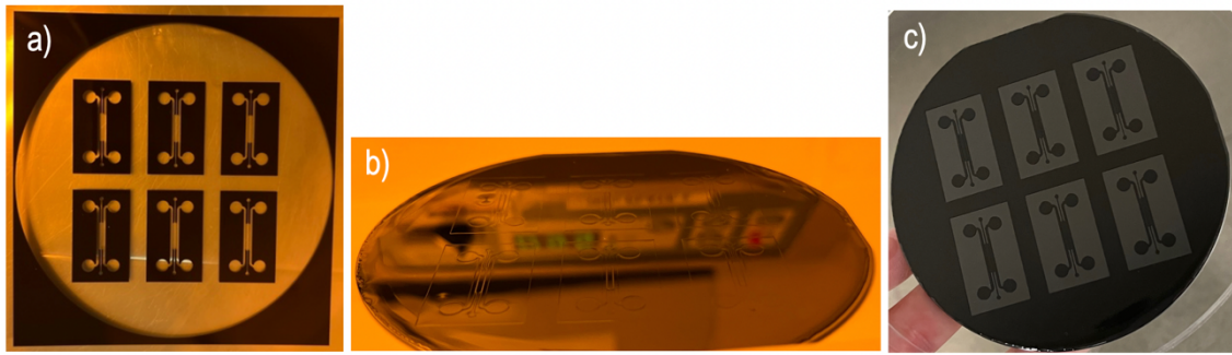
Figure 39: Microchannels molds fabrication results. a) Pattern of acetate mask. b) Pattern on the silane wafer after the UV exposure and the resin detachment. c) Final resulting pattern on the silane wafer after de salinization.
