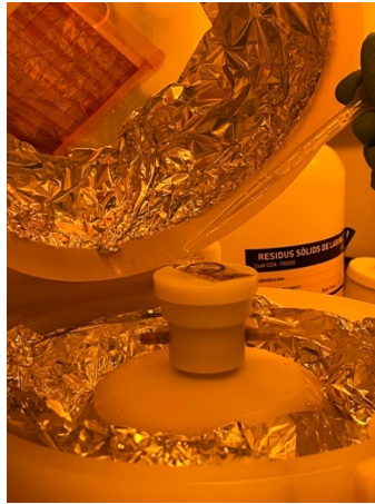
Resin deposition on the coverslip inside a spinner machine.
