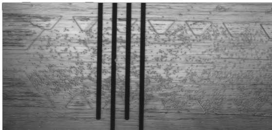
Figure 47: Cells seeded inside a PLA-fibered microchip.
