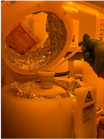
Resin deposition on the coverslip inside a spinner machine.
