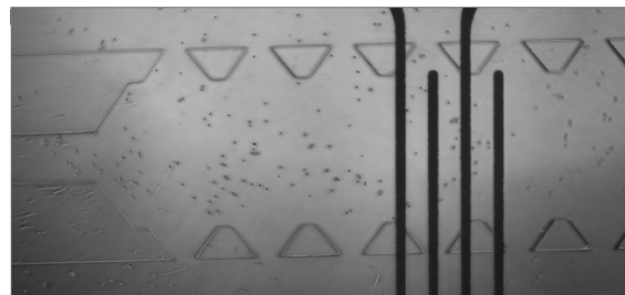
Figure 48: cells seeded inside a fibronectin-filled microchip
