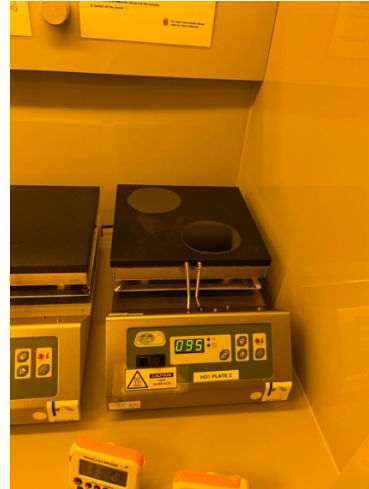
Wafers on a 95°C hot plate
