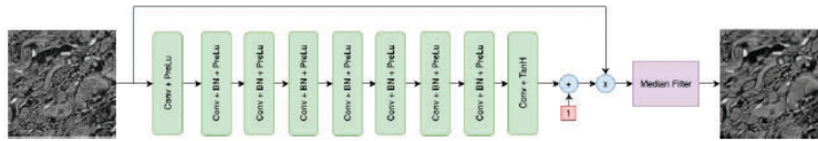
Figure 3: Architecture of the despeckling neural network used in our experiments.
