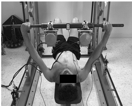
Figure 2. Accelerometer at the center (C) of the bar during isometric extended position (EP).
