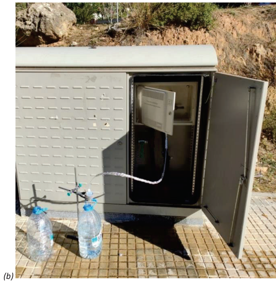
FIGURE S-1. Sampling filter holder (a) and picture of the sampling set-up in the drinking water cabinets (b).
