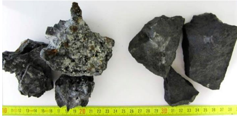
Figure 4. Pictures of raw EAF slags samples showing their general appearance. Source: [12].
