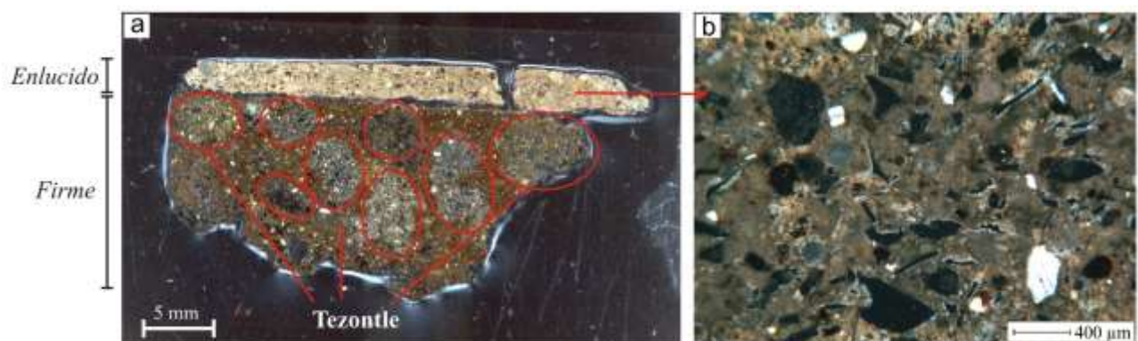
Fig. 2. a) Thin section of sample 53, under crossed nicol, with indication of the enlucido (outer) and firme (inner) layers and the presence of tezontle fragments; b) Microphotographs of sample 53 in thin section, taken using optical microscopy under crossed nicol, with the detail of the enlucido layer including its glass shards.
