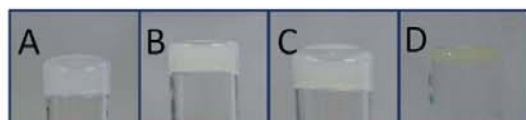
Fig. 2 Gels obtained with the bromide salt of bisimidazolium compound 1 without any drug (A), with sodium ibuprofenate (B), with indomethacin (C) and with the sodium salt of methotrexate (D); ethanol–water proportions are 40 : 60 (A–C) and 45 : 55 (D); 1 : drug ratio (mol/mol) are 2.5 : 1, 4 : 1 and 10 : 1, respectively.
