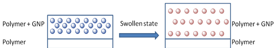
Figure 3.7: Example of gel with embedded GNP. Upon swelling of the gel, the distance between the GNP increases.
