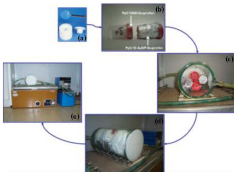
Figure S8. Stages of the experimental set-up of the dynamic dialysis for the ibuprofenate diffusion evaluation: Dichloromethane solutions of 3 \cdot \text{AuNPs} -ibuprofenate complex, 3 \cdot 2\text{Br} -ibuprofenate complex (as control) and 3 \cdot \text{AuNPs} (as control), were placed in biodialysers (a) with one end cap covered with dialysis membrane and closed. Five replicas were prepared for 3 \cdot \text{AuNPs} -ibuprofenate complex to obtain a reproducible measure. The solvent was allowed to evaporate and Milli-Q water (0.8 mL) was added in every biodialyser, which were closed on the other end with a dialysis membrane. Every biodialyser was placed on a closed container with 25 mL of MilliQ-water as receptor phase (b), those with \text{AuNPs} were covered with aluminium foil. All the containers were placed inside a reactor with a water jacket (c) which kept the dialysis systems at 32^\circ\text{C} by using a circulating water bath with temperature control (d). The whole set-up was on a platform with a constant horizontal shake (e).
